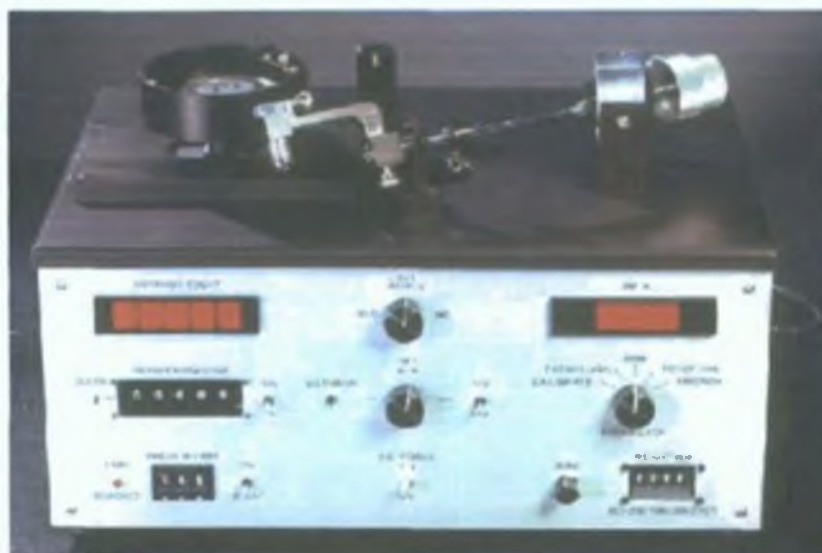
Figure 3.36: Implant Science Corporation ISC-200PC Tribometer (Pin-on-disk) for friction measurement
