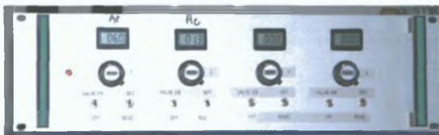
Figure 3.14: Gas flow controller of the deposition chamber
