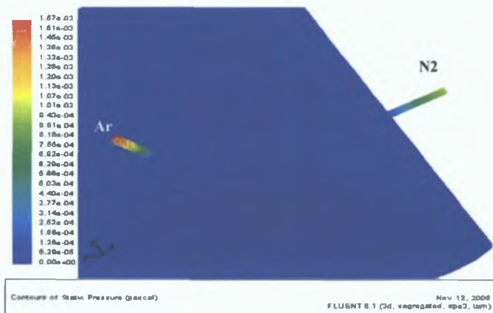
Figure 4.3: Pressure contour of the chamber
