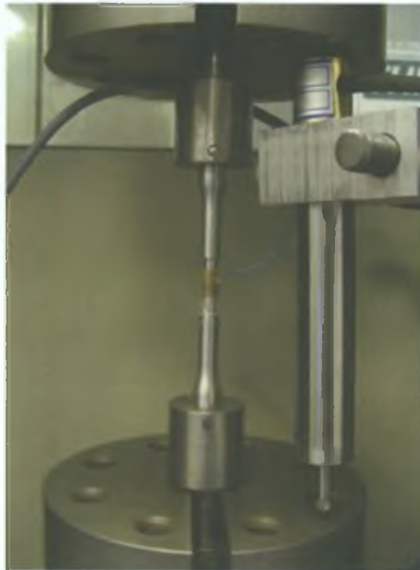
Figure 4.11 AlSiC MMC rod fixed in machine grippers with instrumentation
