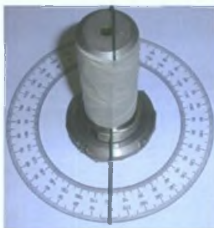
Figure 4.6 Angular position transducer calibration setup
