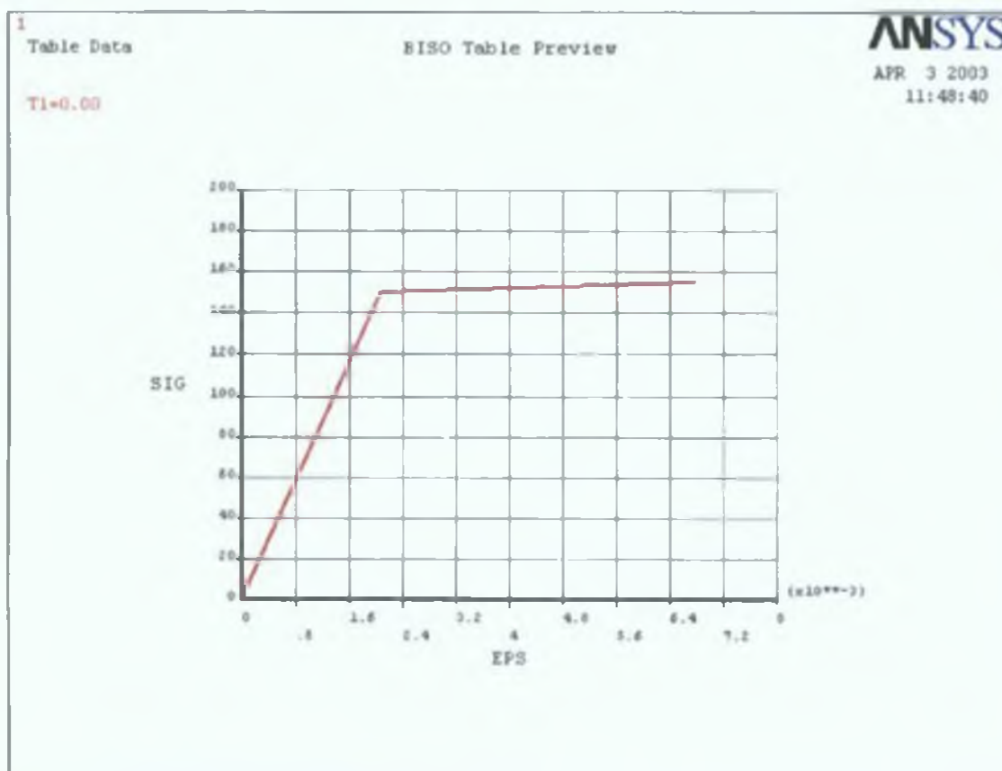
Figure 4.26 Bilinear Material Model for Aluminium matrix
