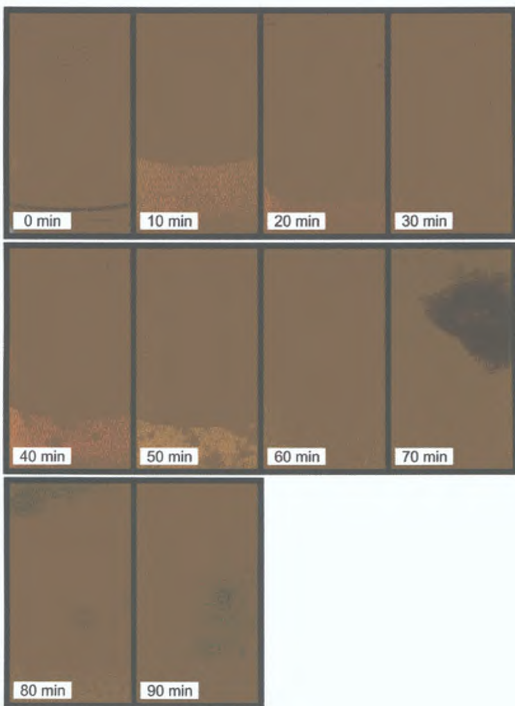
Fig.3.22 - Phase separation of quercetin MIP during processing from t=0\text{min} (prior to initiation of the polymerization) to t=90\text{min} . Initial composition: 15\text{ cm}^3 acetone, 0.05\text{ g} AIBN, 1\text{ mM} quercetin ( 0.338\text{ g} ), 8\text{ mM} 4-vinylpyridine ( 0.8505\text{ cm}^3 ), 40\text{ mM} EGDMA ( 7.544\text{ cm}^3 ).
