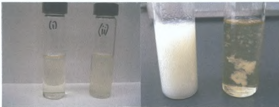
Figure 4.16 – Pre-polymerisation mixtures of 2,4-D MIPs in water/ methanol (i) and chloroform (ii). Greater ‘clustering’ of complexes is evident in mixture (i) – the photo on the right shows both mixtures after heating to 60°C in a water bath for 15 minutes.
