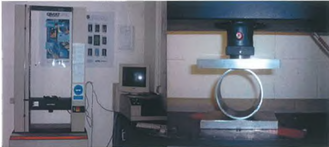
Figure 4-1: Instron Machine and a sample specimen.
