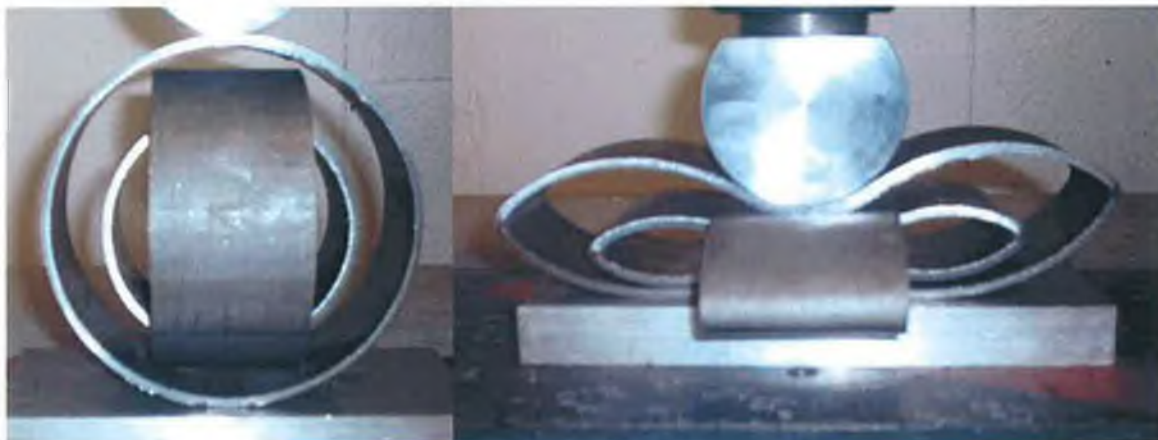
Figure 5-9: Initial and final stages of deflection for a COPSS crushed under a cylindrical indenter.
