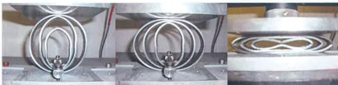
Figure 5-24: Initial and final stages of compression for an OIPSS. [Compression method]
