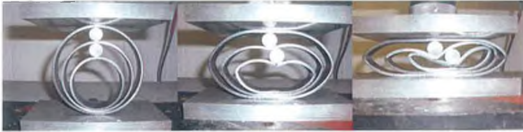
Figure 5-18: Initial and final stages of compression for a CIPDS. [Sample 1]
