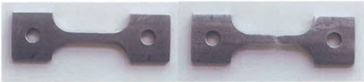
Figure 4-11: A sample tensile specimen before and after tensile loading.
