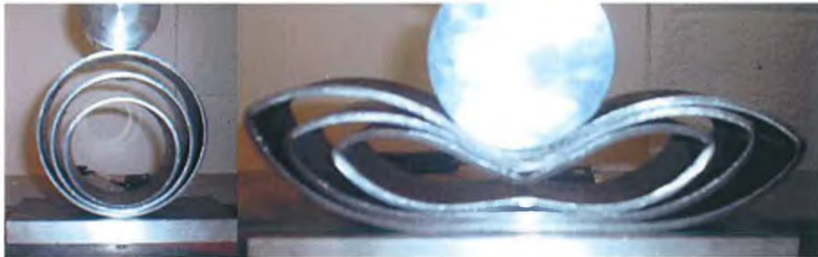
Figure 6-18: Initial and final stage of deflection for a CIPSS with no constraints.
