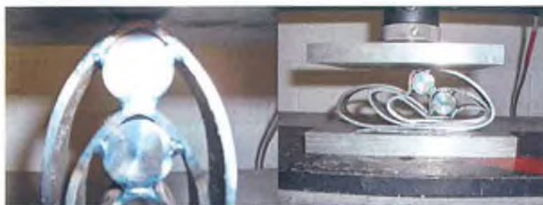
Figure 5-25: The initial and final stages of compression for an OIPDS with spot welds. [test 3]
