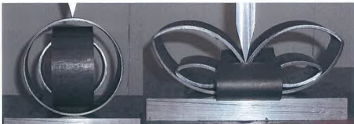
Figure 5-6: Initial and final stages of deflection for a COPSS crushed under a point load indenter.
