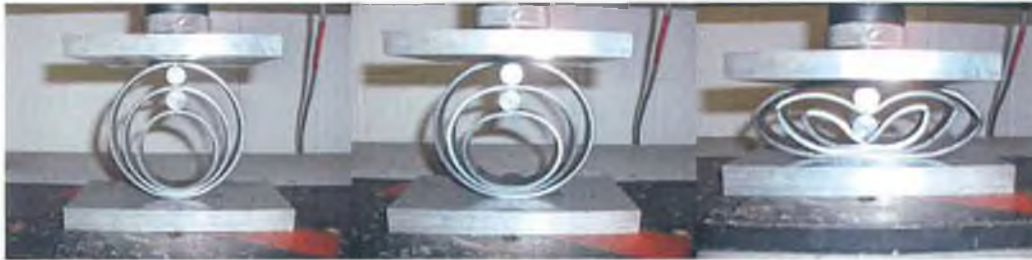
Figure 5-20: Initial and final stages of compression for a CIPDS. [Sample 3]
