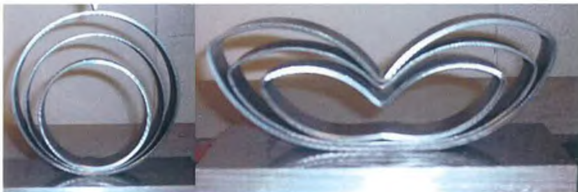
Figure 6-10: Initial and final stage of deflection for a CIPSS with no constraints.
