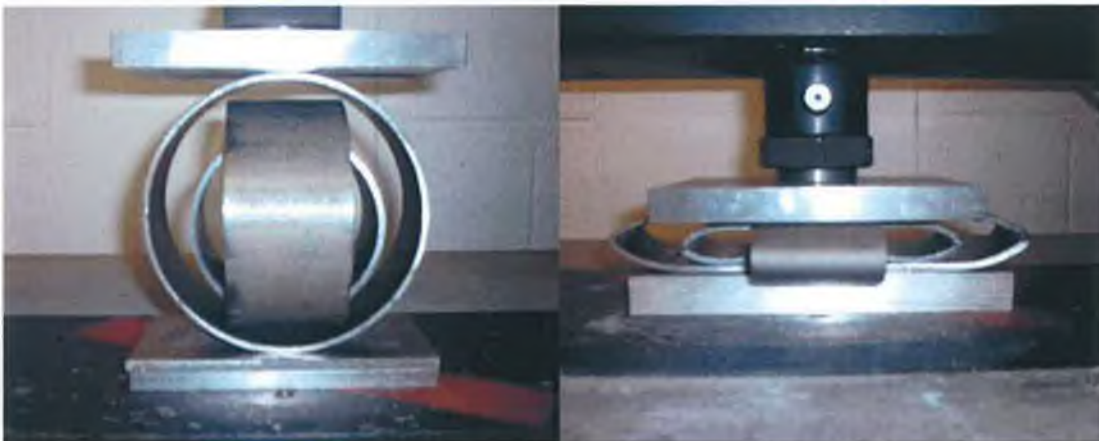
Figure 5-4: Initial and final stages of deflection for a COPSS crushed under a rigid flat platen.
