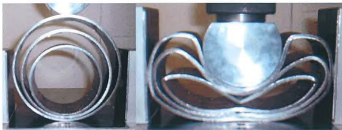
Figure 6-22: Initial and final stage of deflection for a CIPSS with vertical constraints.
