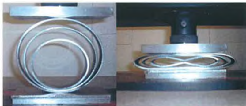
Figure 6-2: Initial and final stage of deflection for a CIPSS with no constraints.
