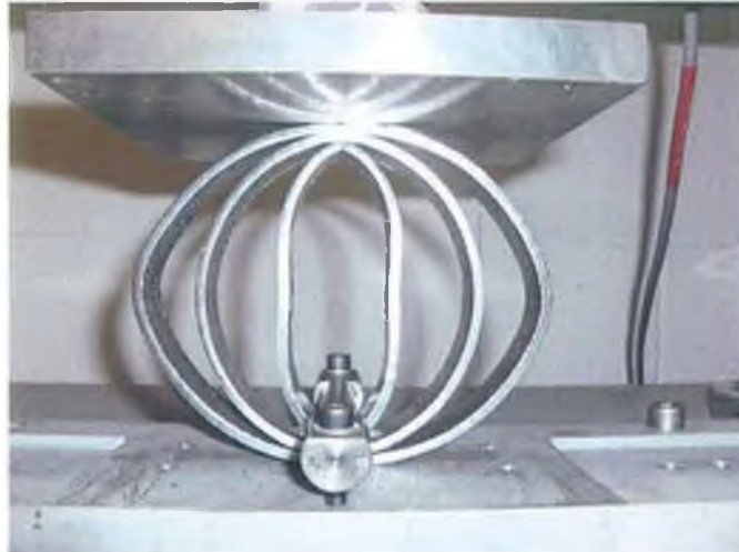
Figure 4-5: The fixture used to hold the samples in place upon impact.
