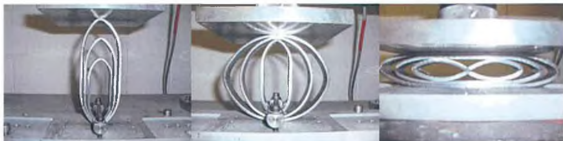
Figure 5-22: Initial and final stages of compression for an OIPSS. [Tension method.]
