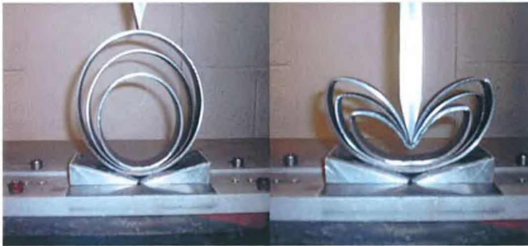
Figure 6-12: Initial and final stage of deflection for a CIPSS with inclined constraints.
