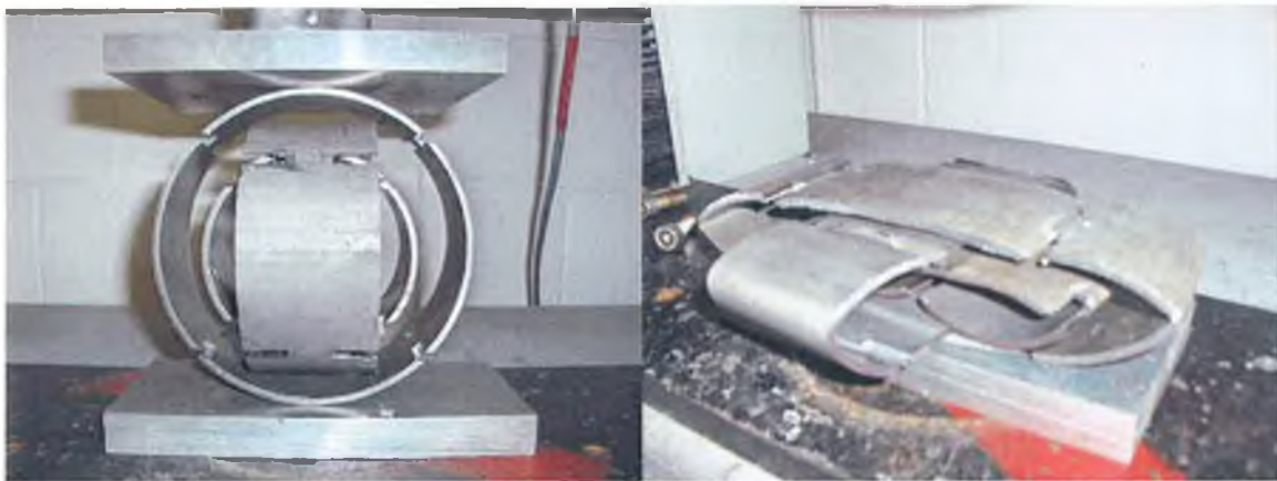
Figure 5-13: Initial and final stages of deflection for a SCOPSS. [Sample 1]
