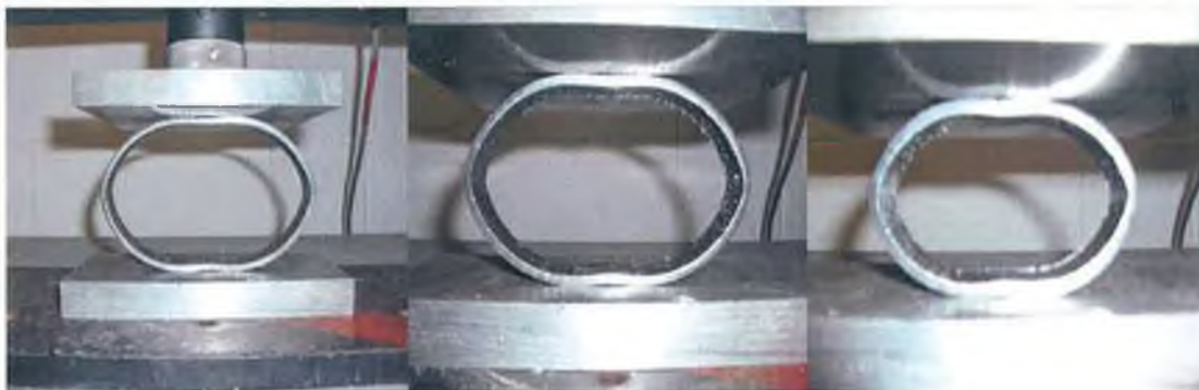
Figure 4-7: The final stages of displacement for each tube using the compression method.
