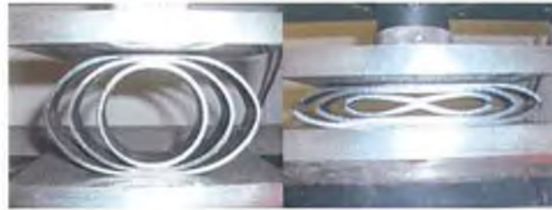
Figure 5-1: Initial and final stages of compression for a CIPSS.
