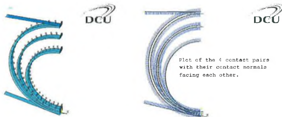
Figure 7-68: A graphical plot of the boundary conditions and contact pairs for a CIPSS with inclined constraints.
