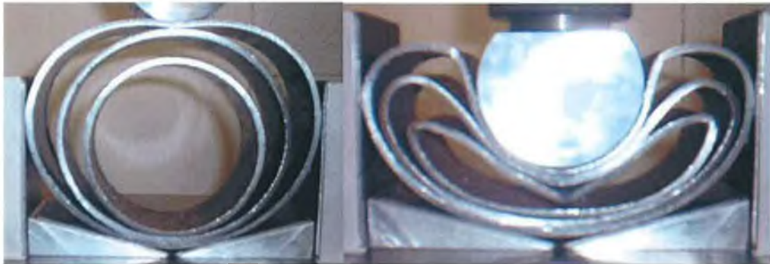
Figure 6-24: Initial and final stage of deflection for a CIPSS with both constraints.
