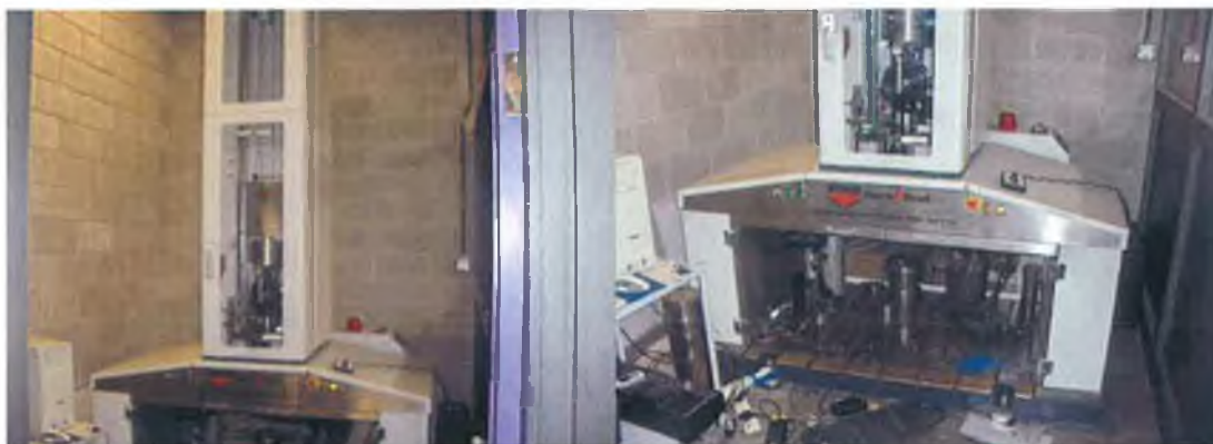
Figure 4-2: Photographs displaying the Zwick Roell 5HV series used to conduct the impact experiments.
