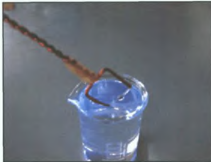
Figure 3.33 Manual dip coating of chip thermistor probe. The entire probe is fully immersed in the coating material and is then withdrawn slowly. Note that the sensor is oriented at an angle in relation to the surface of the bath. If this were not the case then the coating material would break away from the sensor abruptly and leave a globule of coating on the sensor, which would dramatically affect its performance.
