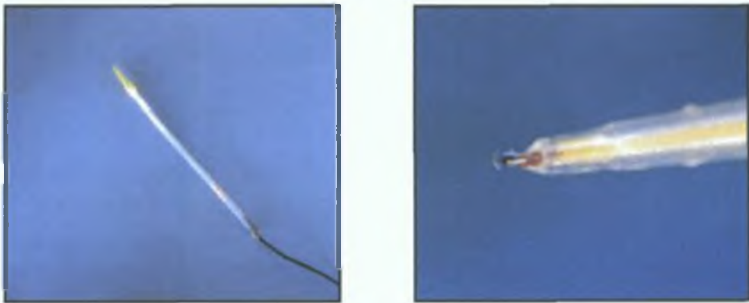
Figure 3.27 Glass Bead Thermistor Sensor. The thermistor is mounted in a rigid conical plastic tube. Insulation at the bead/tube interface is achieved using cyanoacrylate-based adhesive. This assembly is then connected to a semi-rigid nylon tubing, through which the connecting cable passes.
