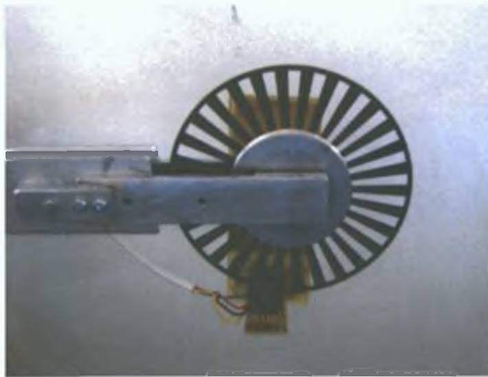
Figure 3.19 Optical chopper and slotted opto-switch assembly. In this picture it is located on Pulley 2 (see Figure 3.23). As the chopper rotates the slotted opto-switch gives out a series of voltage pulses that are ttl compatible, allowing the signal to be connected directly to a PC or other digital device for analysis.
