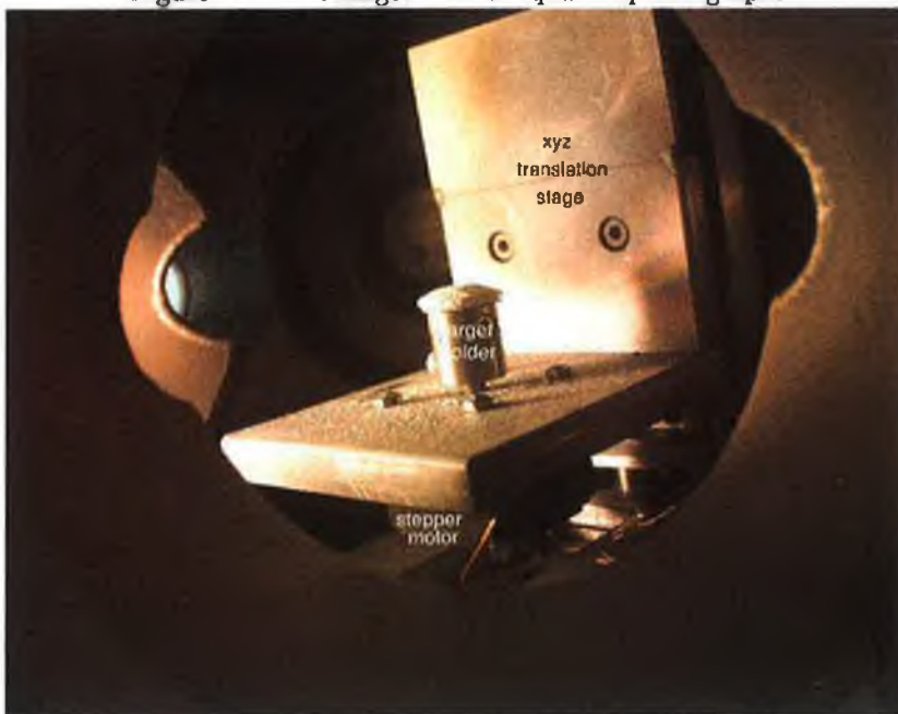
Figure B.5: A view of the target holder, translation and rotation setup.
