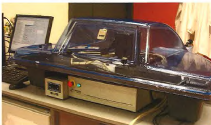
Figure 7.15: Genomic Solutions array printing system used for deposition of sensor films.
