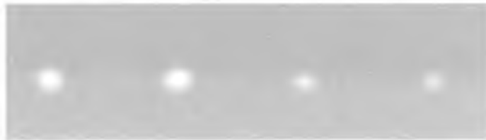
Figure 9.1: Image of fluorescence from a 4-channel UV curable sol-gel waveguide platform at 0% oxygen.
