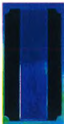
Figure 6.13: Fluorescence intensity image from PMMA-OH-NH 2 -Cy5 (only bottom portion of slide modified), recorded using a Genetics Microsystems 418 fluorescence scanner.
