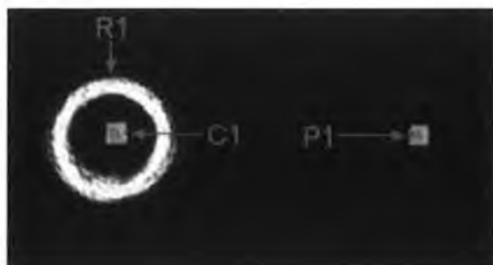
Figure 5.7: A representative image of the fluorescence intensity recorded from an enhancement chip. The ring and spot on the left-hand-side of the image corresponds to the fluorescence recorded from doped sol-gel printed on the top of a frustrated cone. The spot on the right-hand-side of the image corresponds to the fluorescence recorded from doped sol-gel printed on the planar portion of the chip.
