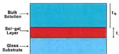
Figure 5.8: Schematic of multilayer system, consisting of a glass substrate, sol-gel layer and bulk layer.
