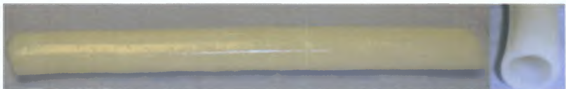
Figure 5.5 Sample PVA-chitosan hydrogel vessel. The vessel was fabricated from PVA and chitosan solutions blended at a ratio of 3:2, then crosslinked using a combination of freeze-thaw cycles and submersion into a potassium sulphate coagulation bath.
