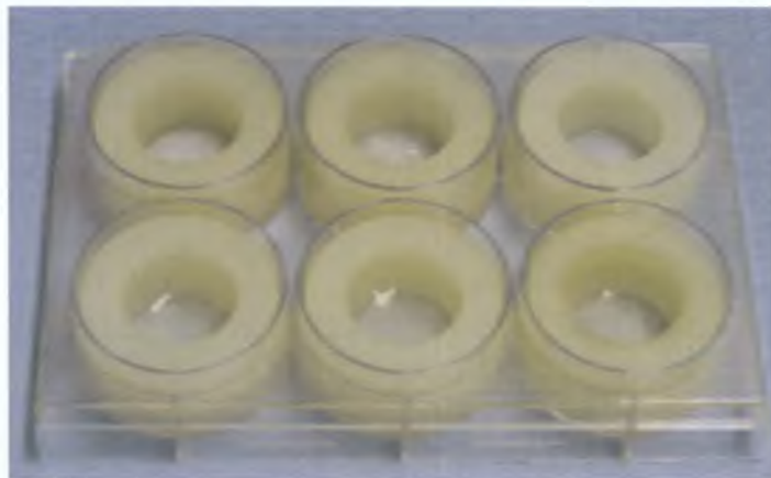
Figure 4.7 6-well culture plate with membranes and nylon inserts.
