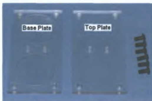
Figure 5.3 Mould for manufacturing PVA-chitosan bi-axial membranes.
