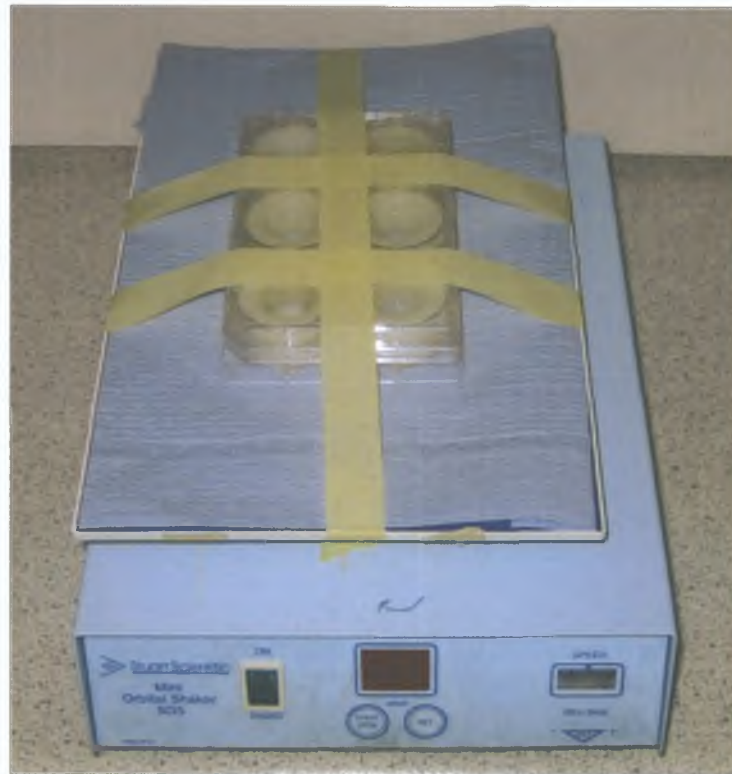
Figure 4.10 6-well culture plate was secured to the orbital shaker.
