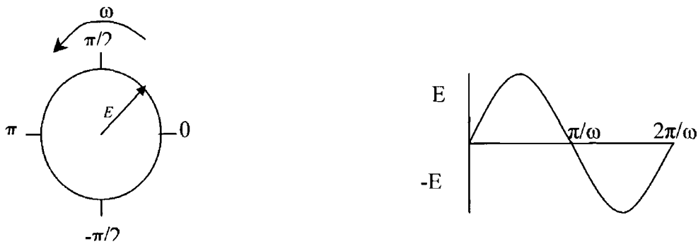
Figure 4.5.1 Sinusoidal voltage displayed as phasor quantities
