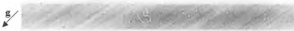
Figure 13.5: Section transmission topograph from 1\bar{1}\bar{1} reflection of sample FZ-NIST. No Pendellösung fringes are seen in the image as only the branch one wavefield propagates within the crystal.
