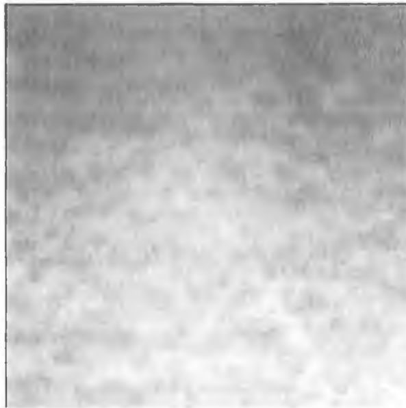
Figure 12.2: 115 total external reflection topograph for sample SiGe 774. Incidence angle \alpha_o = 0.05^\circ . Scattering depth \Lambda = 1.29 \text{ \AA} .
