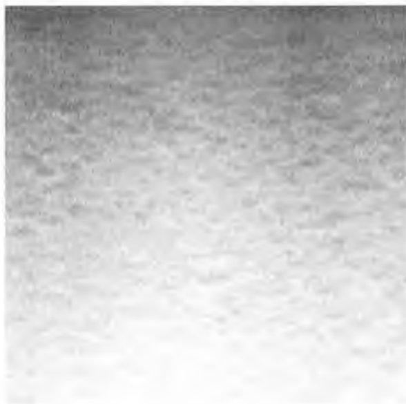
Figure 12.3: 115 total external reflection topograph for sample SiGe 775. Incidence angle \alpha_o = 0.05^\circ . Scattering depth \Lambda = 1.29 \text{ \AA} .
