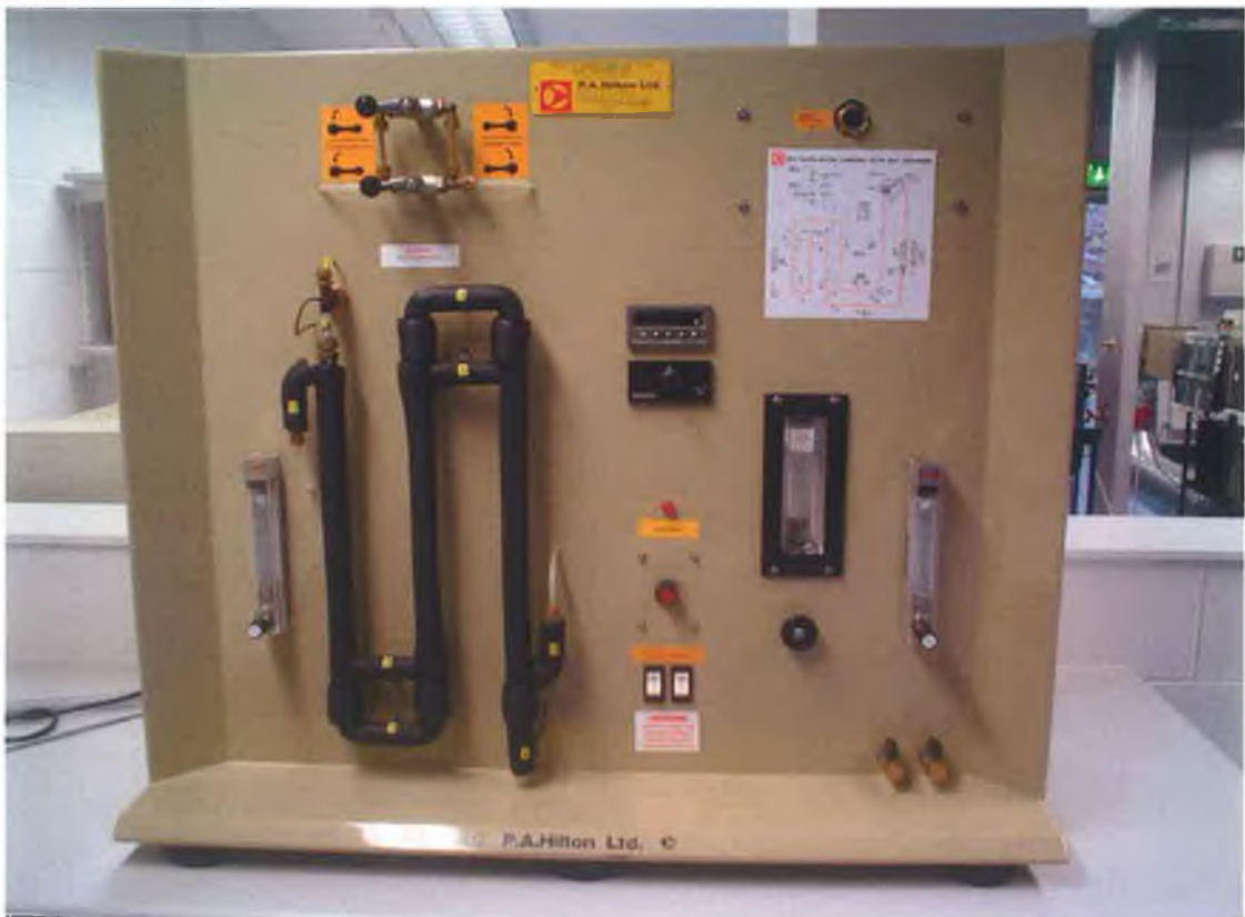
Photo 3.1 Existing heat exchanger
