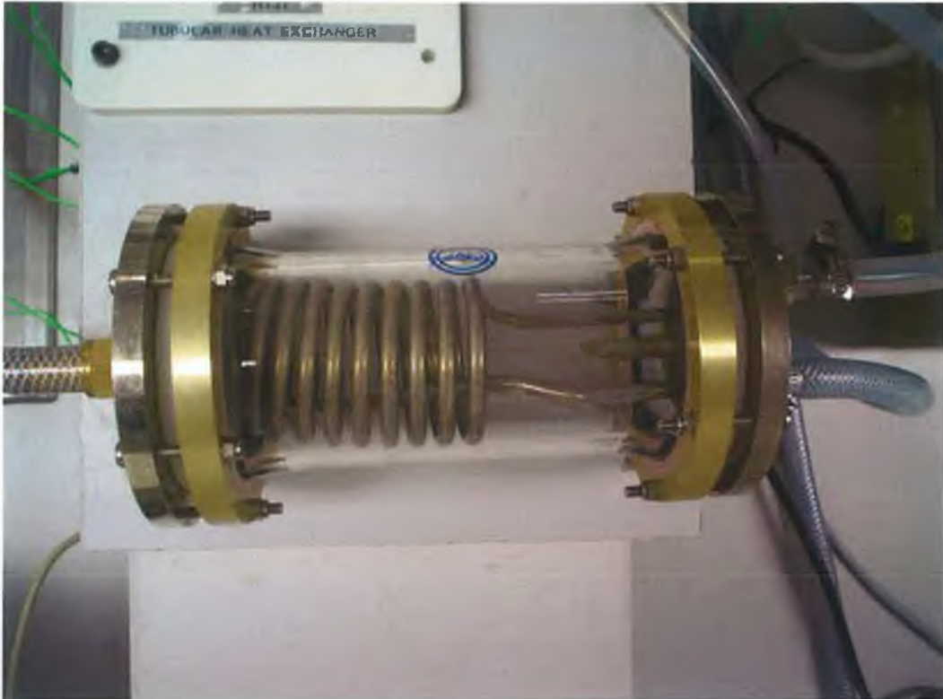
Photo 3.4 New cooling system
