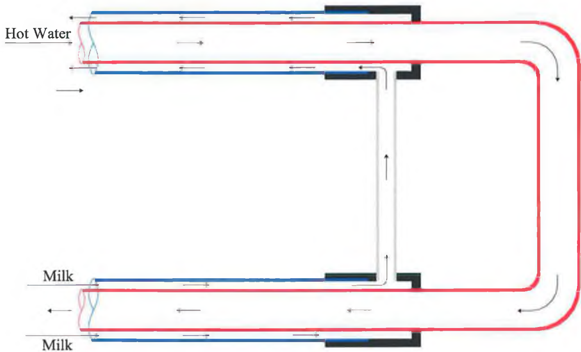
Fig. 2.5.2 Flow arrangements through the hairpin fittings
