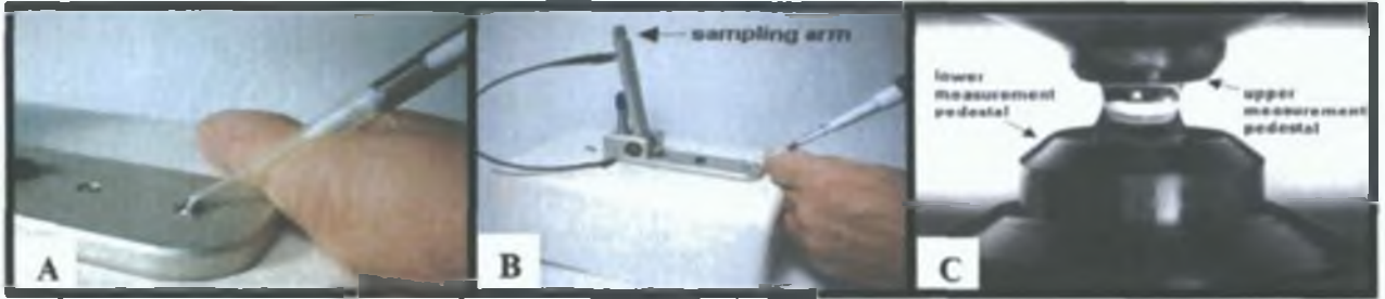
Figure 2.9.1.1 Samples are quantified by loading 1µl onto the receiving fibre (A), the source fiber, connected to the sampling arm (B) is brought down into contact with the sample allowing a 1mm gap between the upper and lower pedestal (C), through which the light is passed. (Pictures adapted from ND-1000 Spectrophotometer users manual V 3.1.0).
