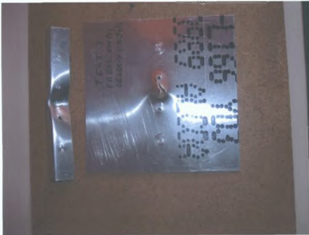
Figure 5.5: Test plate 7 with petalling of plate with tearing, failure of all four rivets but no perforation of angle. Initial velocity 218m/s
