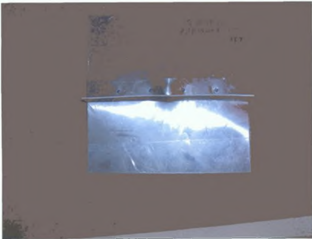
Figure 5.3: Test plate 4 with no perforation of angle and no rivet failure. Initial velocity = 162m/s
