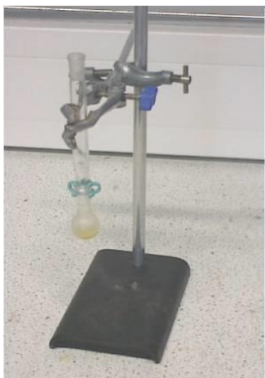
Figure 3: Microscale apparatus for preparation of soap using air condenser
