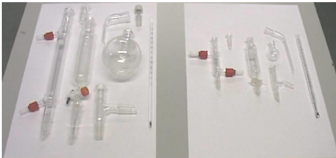
Figure 1: Conventional and Microscale apparatus for organic synthesis
