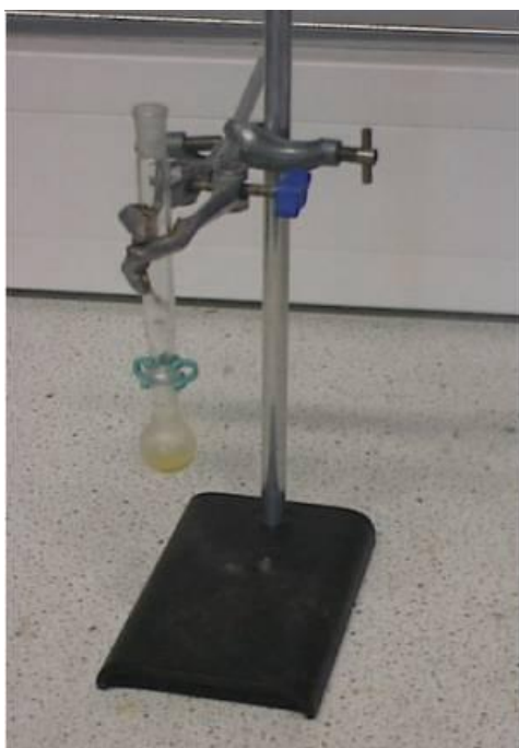
Figure 5.4: Air condenser for the preparation of soap on a microscale
