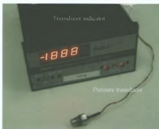
Figure 2. 5: Pressure transducers and Transducer indicator unit
