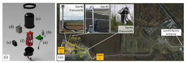
Figure 1: (i) Exploded view of platform (a) microcontroller (MSP430), (b) sensors, (c) IP68 casing, (d) battery, (e) GSM module, (f) extraction pump. (ii) Configuration of wireless sensor network deployed on landfill site.
