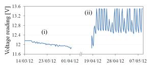
Figure 2: Power levels during operation (i) battery depletion rate, (ii) battery solar recharging
