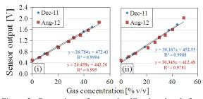
Figure 3: Comparison of sensors' calibration data before and after 8 months deployed (i) CO<sub>2</sub>, (ii) CH<sub>4</sub>.
