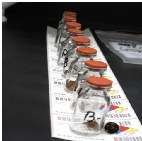
Figure 5.27, Collected corrosion products.
