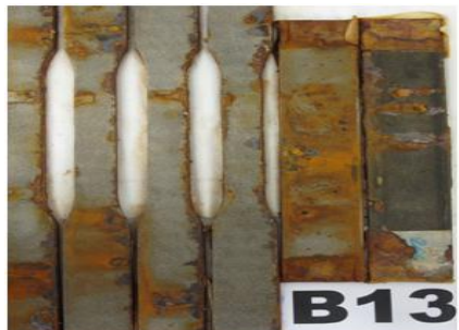
Area Failed % 11 To 20= Rating No. 5
