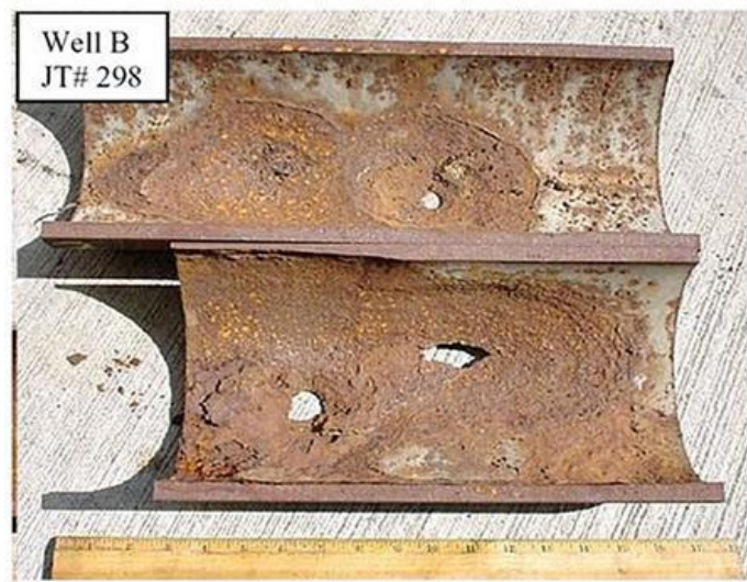
Figure 1.1, Sour gas well production pipe failure due to localized corrosion [3].
