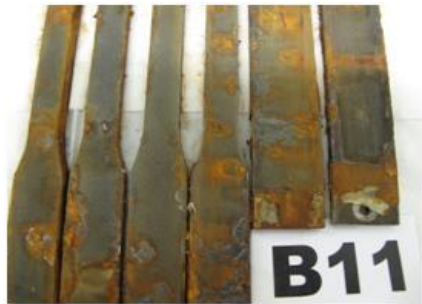
Area Failed % 21 To 30= Rating No.4
