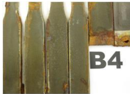
Area Failed % 2 To 3= Rating No.8
