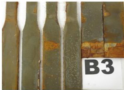
Area Failed % 2 To 3= Rating No.8
