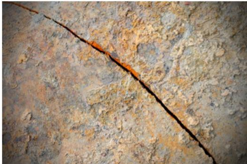
Figure 1.3, Hydrogen Induced Cracking (HIC) occurs when carbon steel is exposed to hydrogen sulphide (H 2 S) [6].
