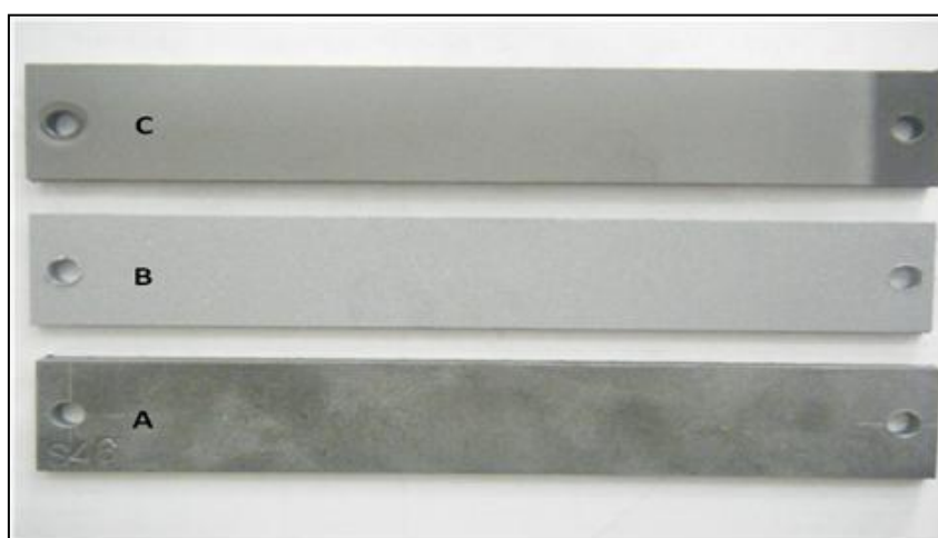
Figure 3.22, Test Specimens: (A) Base metal, (B) After grit blasting, and (C) After multi-layer coating applied.
