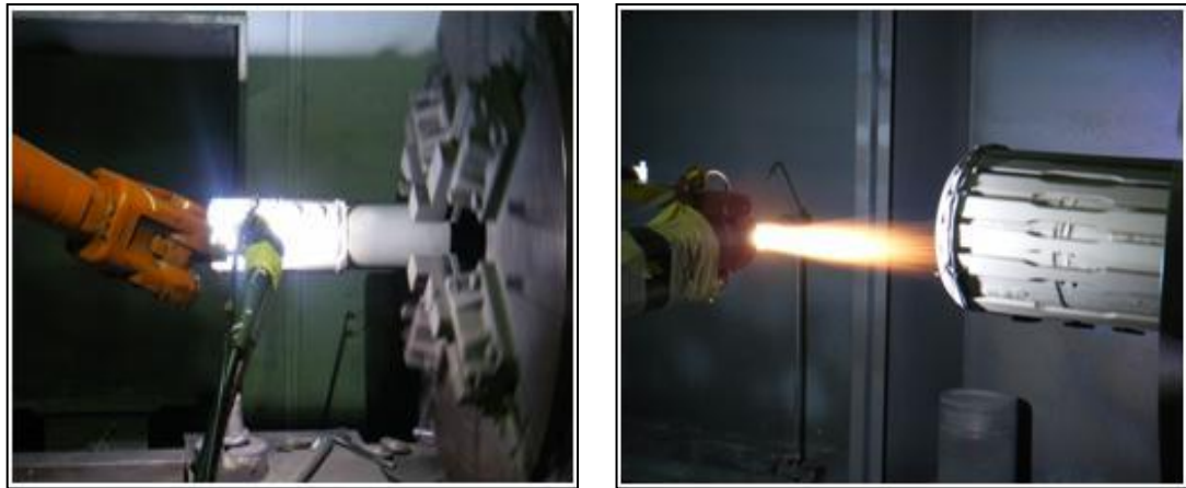
Figure 3.20, Plasma thermal spraying coating process used in this research.
