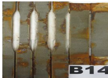
Area Failed % 11 To 20= Rating No. 5
