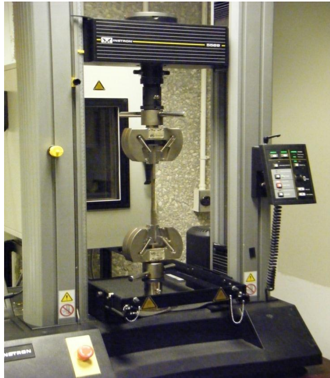
Figure 3.41, Photograph of the Instron tensile testing machine with sample attached.
