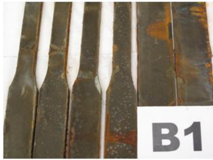
Area Failed % 4 To 6= Rating No.7
