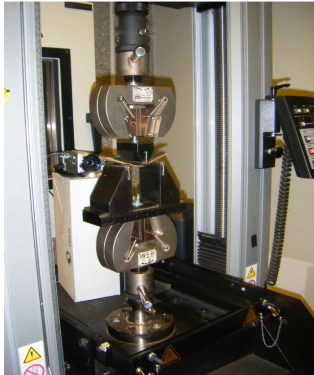
Figure 3.38, Instron testing instruments used for three point bending test
