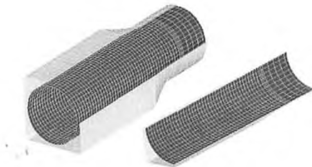
Fig 2.4.3 3D finite element model of the tube and die [69]
