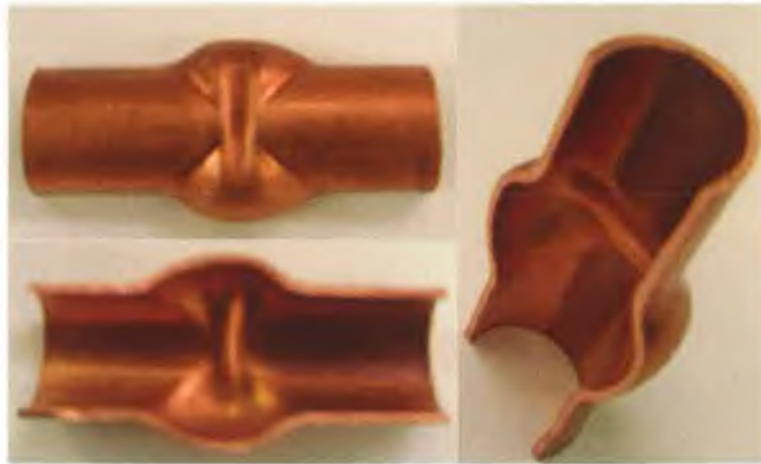
Fig 3.4.32 Wrinkle growth at the centre of the tube for a X-branch expansion
