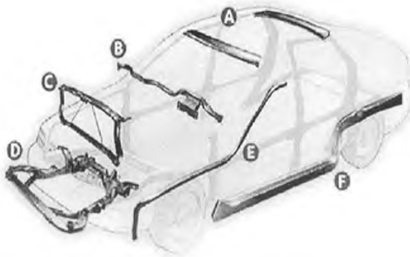
Fig 1.1.2 Automotive application of hydroforming- A. roof headers, B. instrument panel support, C. radiator support, D. engine cradles, E. roof rails, F. frame rails [2]
