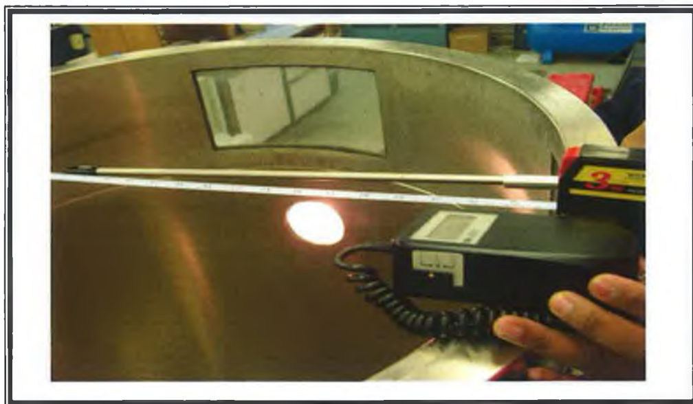
Figure 3.8: Air nozzle velocity measured at the top of the spray dryer by electronic potentiometer.
