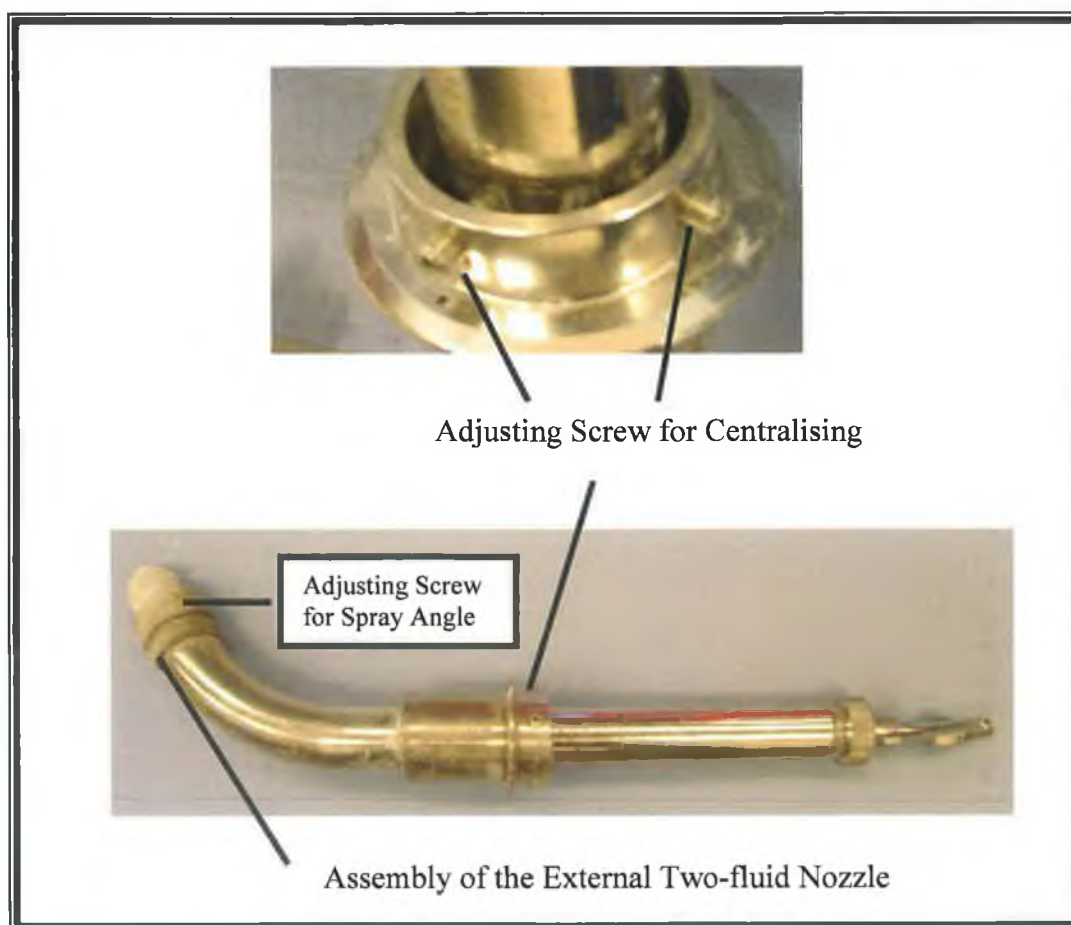
Figure 3.5: Assembly of the external two fluid nozzle with adjusting screw to set the spray angle.
