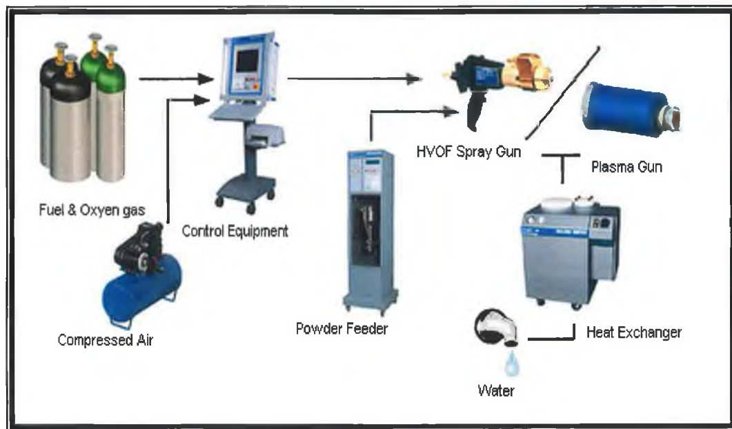
Figure 2.13: Equipments involved in the plasma thermal spray process [104].
