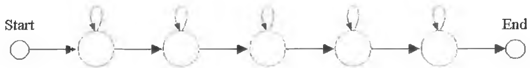
Figure 2.6: A sample DHMM topology with seven states including the start and end states.
