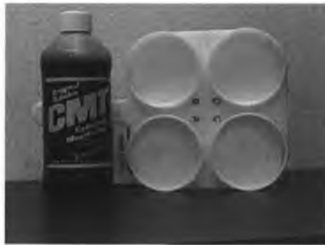
Figure 1.7: The equipment required to perform a CMT test (bottle of reagent and paddle).
