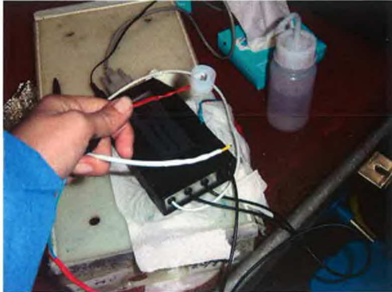
Figure 5.12: Photographs of the new prototype impedance device.
