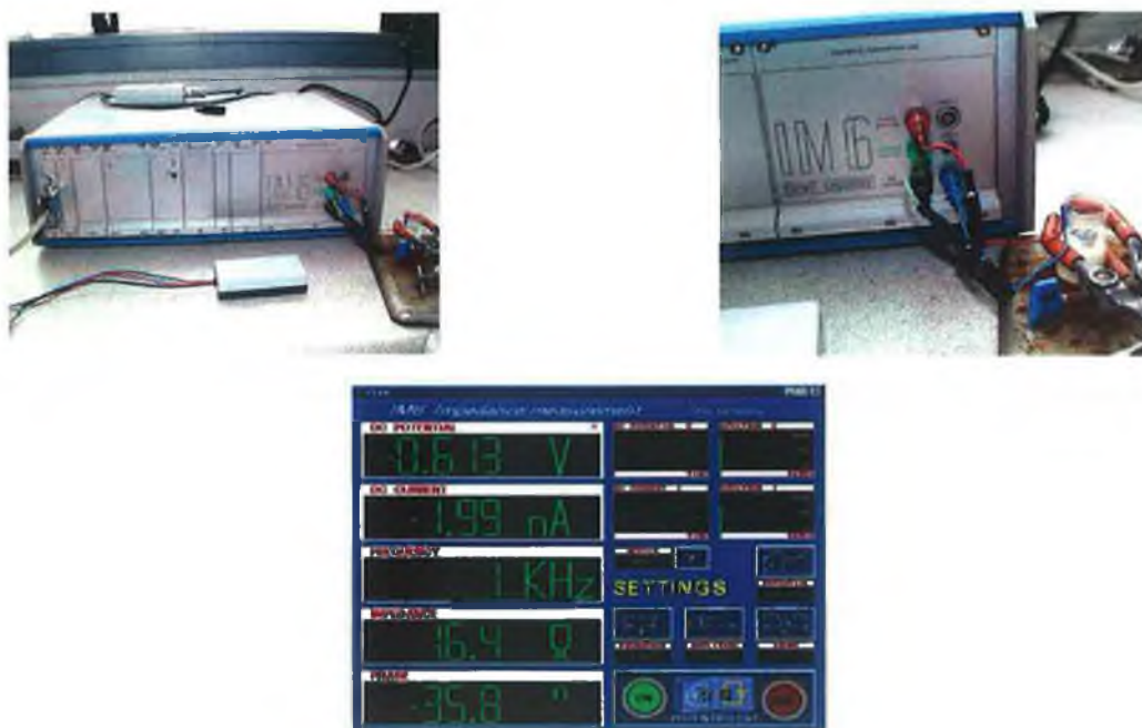
Figure 3.2: Photographs of the instrumentation for EIS measurement at high frequencies IM6 d and its software Thales®.
