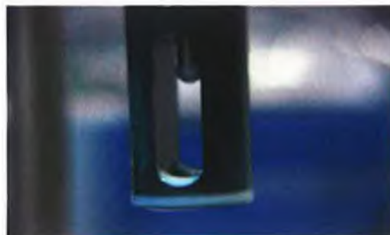
Figure 3.8: Conductivity cell after measurement; milk residue remains in the temperature probe, the graphite electrode and on the plastic body.
