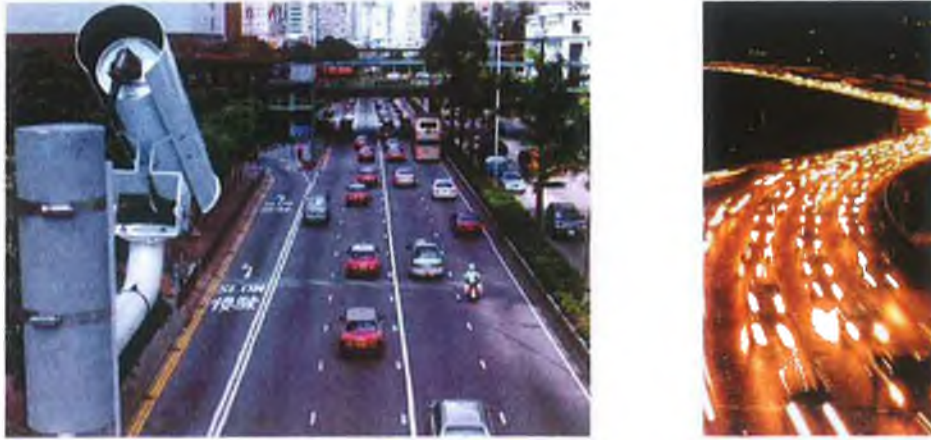
Figure 2.3: (a) Autoscope Solo Pro automatic incident detection in Hong Kong (b) Night image of vehicles to illustrate headlight blooming
