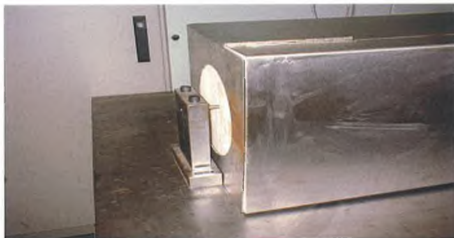
Figure E7 Insulating material surrounded by steel plates, capillary tube and end support for the capillary tube.
