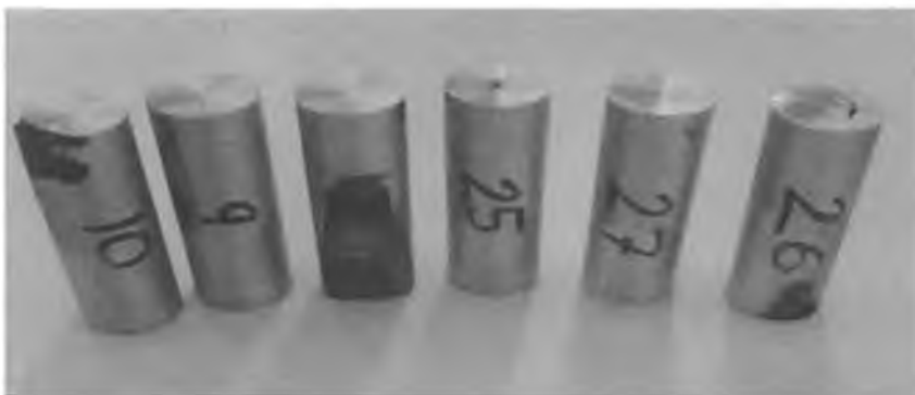
Figure F.3 Images of feedstock billets after finish machining, sample numbers 25, 26, 27 & 8, 9, 10.
