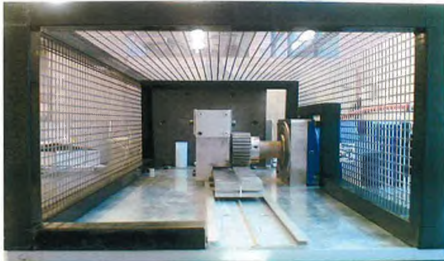
Figure E4 Side view of piston motion mechanism
