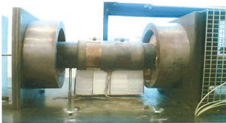
Figure E6 Injection chamber, heater bands, steel rod transmitting pressure to load cell, injection chamber supports and insulation material.
