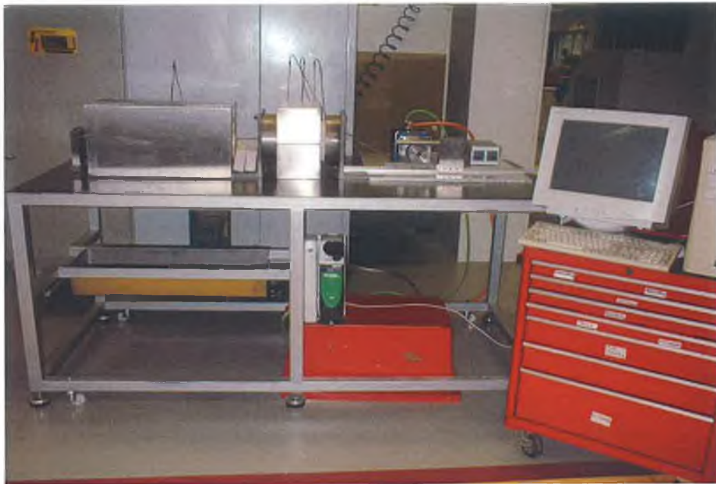
Figure E1 Capillary viscometer developed
