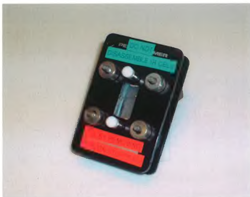
Figure 4.6: NaCl windowed cell for aqueous acetic acid sensing
