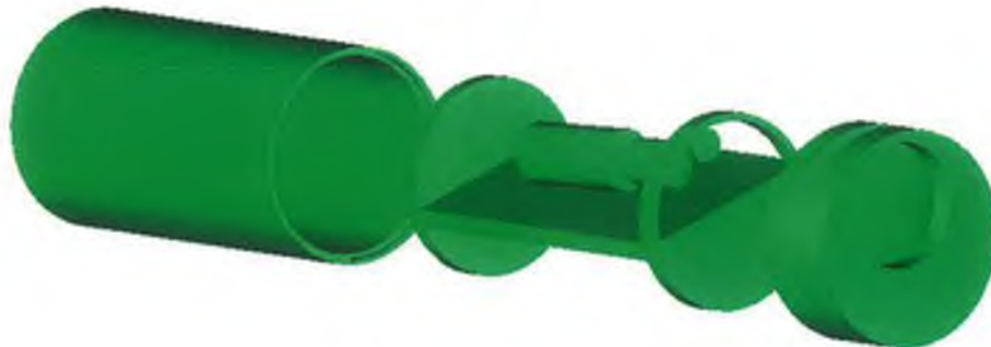
Figure 3.5: 3D view of prototype with outer housing, optical platform and liquid head. The electronics are situated on the bottom of the platform
