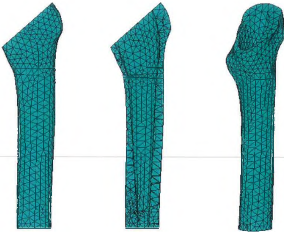
Figure K.3: (Left) Elevation view of meshed femur; (Middle) Elevation view of sectioned femur to reveal internal mesh; (Right) Auxiliary view of meshed femur
