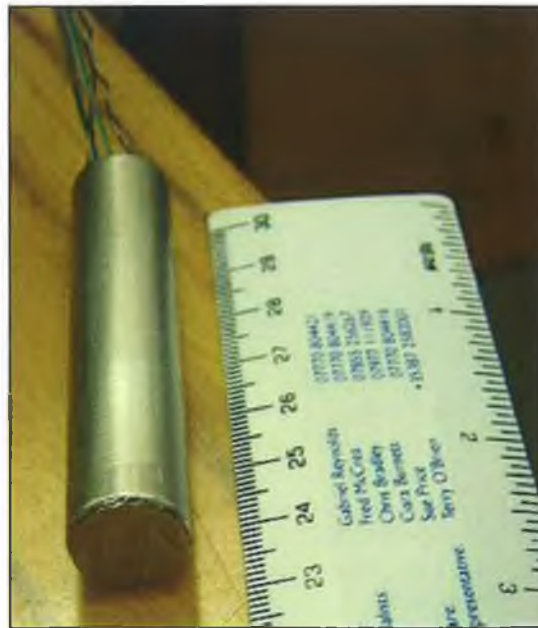
Figure 3.1: 316L stainless steel tube used to represent the femoral prosthesis in the experimental model
