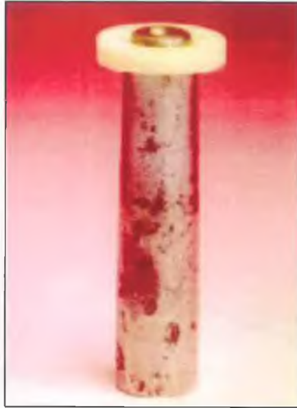
Figure 2.21: No.2 Morse taper mandrel with an acrylic bone cement ring assembled. Reprinted with permission of Orr et al [33].
