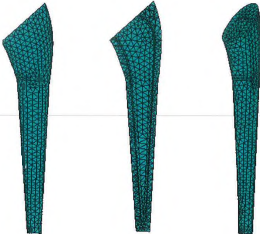
Figure K.2: (Left) Elevation view of meshed cement mantle; (Middle) Elevation view of sectioned cement mantle to reveal internal mesh; (Right) Auxiliary view of meshed bone cement mantle
