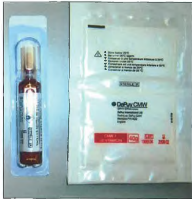
Figure 2.1: Monomer ampoule (left) and polymer packet (right) of CMW ® 1 Gentamicin bone cement
