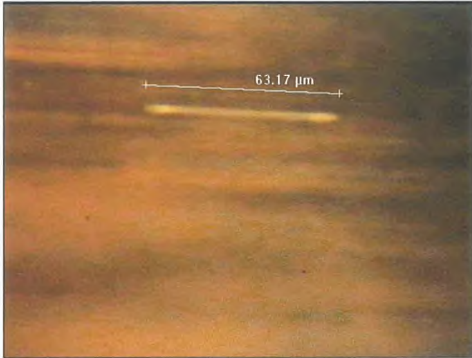
Figure 4.13: Image of internal wire waveguide displacement obtained by the optical microscope and image analysis software. Initial length of mark was 9.2\mu\text{m} and the image streak length of 63.17\mu\text{m} giving a displacement of approximately 54\mu\text{m}
