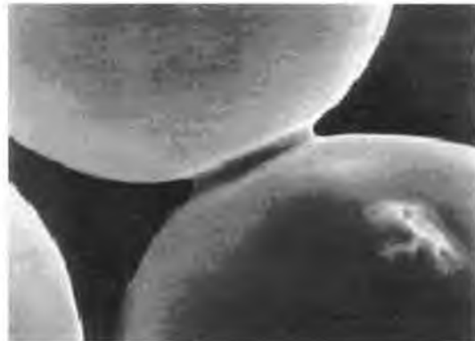
Fig. 1.6: Neck in the point of particle contact.
