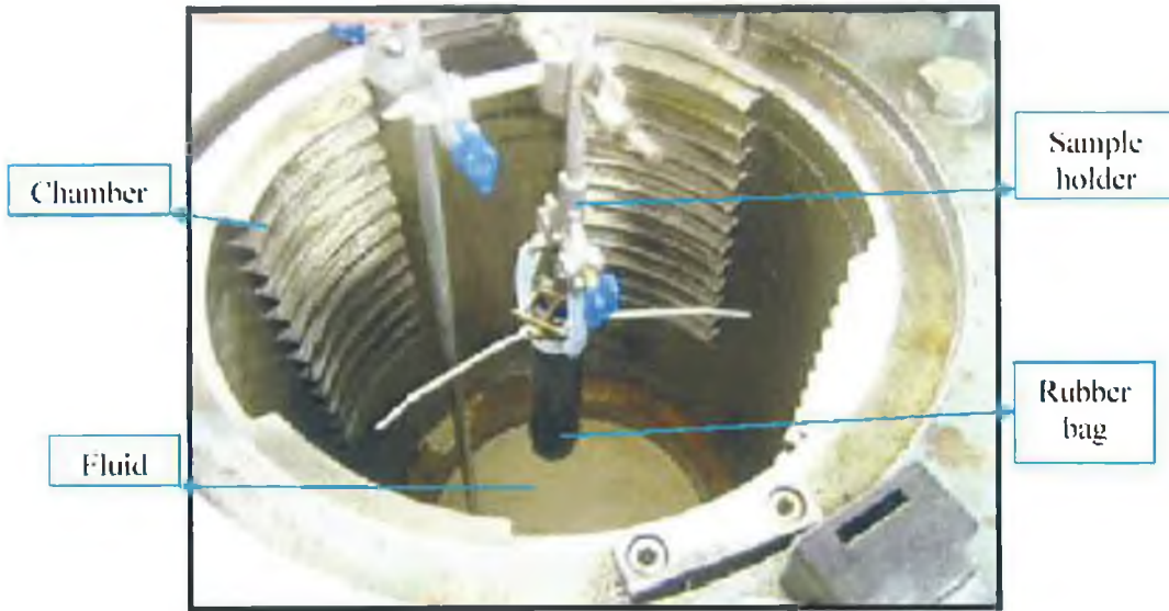
Fig. 3.7: isostatic press.
