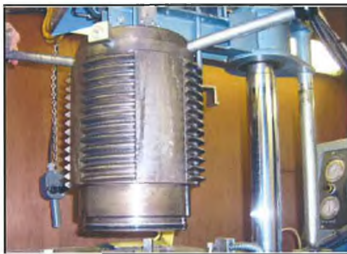
Fig. 3.6: The breech nut of the isostatic press, used to close the chamber.
