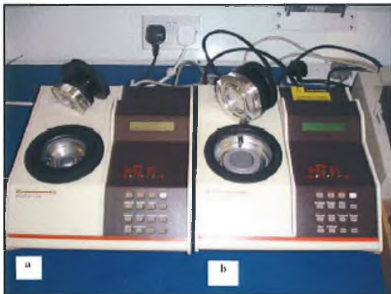
Fig.3.2: Accupyc 1330 pycnometer (a) small volume helium pycnometer and (b) large volume helium pycnometer.
