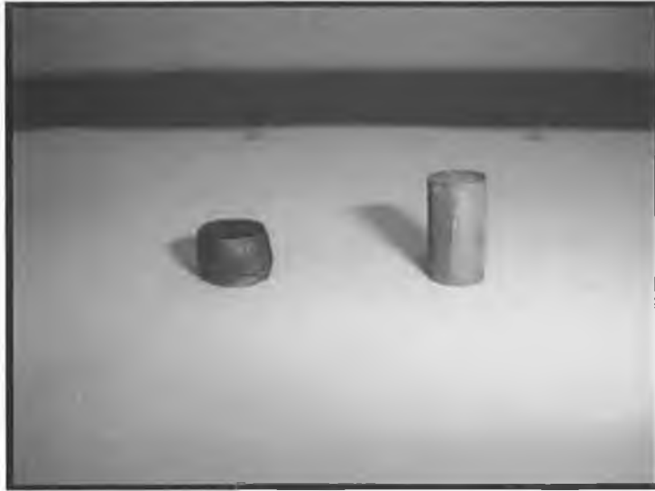
Fig. 3.17: Specimen before testing and after 50% height reduction.
