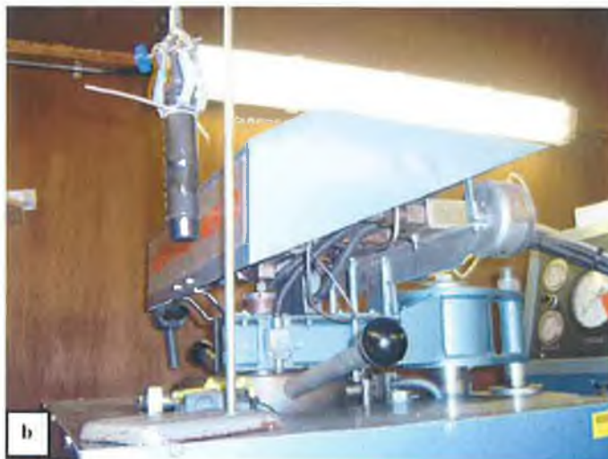
Fig. 3.5: The rubber bag with vacuum tube clamped, over the isostatic pressure chamber.
