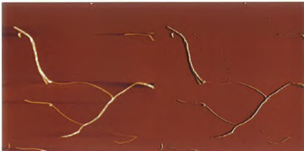
Figure 4.9 7.436\mu\text{m} \times 7.436\mu\text{m} TM-AFM height (left) and amplitude (right) images of MWNT-NH 2 Left: height z = 75\text{nm} , Right: Amplitude z=90\text{mV} .
