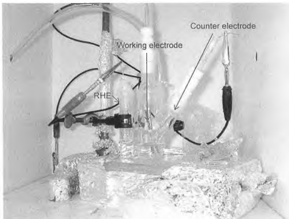
Figure E.2 Electrochemical cell showing (left) the Reversible Hydrogen Electrode (RHE); (middle) the working Au(111) electrode; and (right) the counter electrode.
