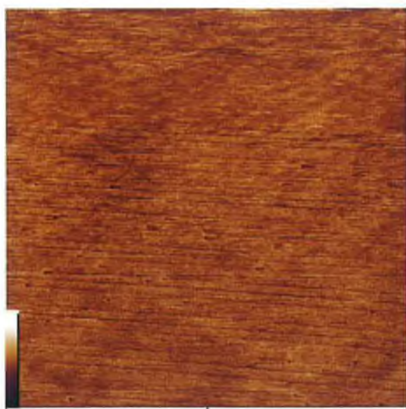
Figure 3.10 5 \mu m x 5 \mu m tapping mode AFM height data of solvent rinsed native oxide covered silicon (100) substrate. The z-range is 2nm.
