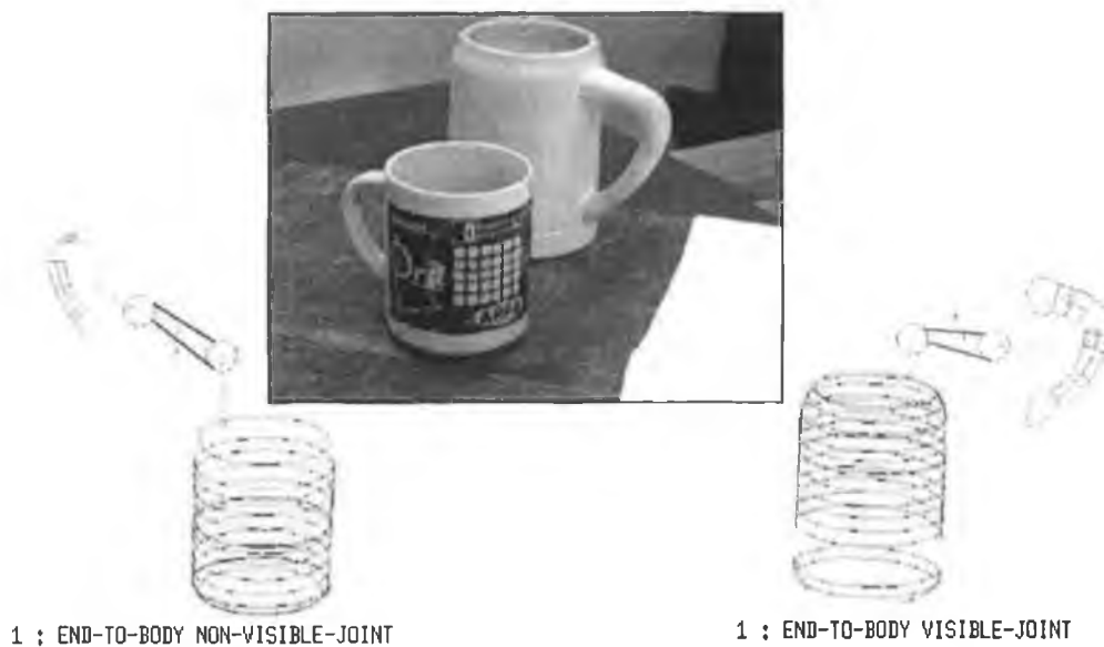
Figure 3.8: Example of pose of an object detected using the process in (Zerroug & Nevatia 1995). Each detected object is described as a graph where nodes are parts and arcs labeled joint relationships between parts.
