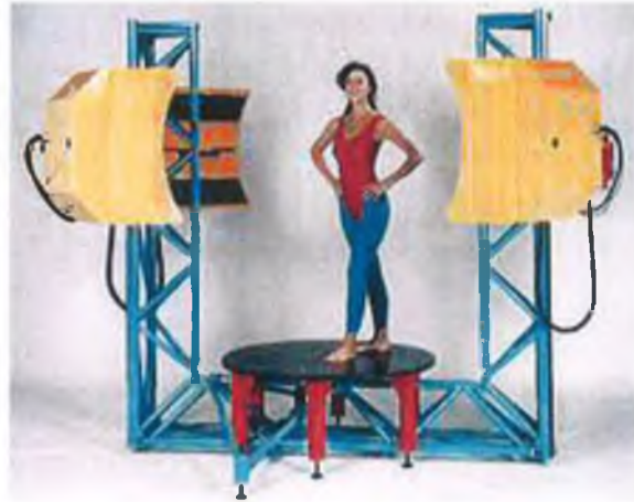
Figure 3.12: The Cybware whole body scanner system 12 .
