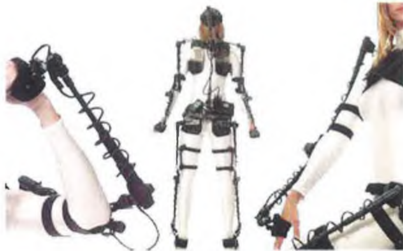
Figure 3.9: The Gypsy Motion capture System is shown. This motion capture system is an electro mechanical system that consist of an exoskeleton made of lightweight aluminium rods that follow the motion of the performer's bones 11 .
