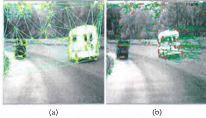
Figure 2.9: Example of the application of active-meshes. (a) shows the generated mesh that is used to track the position of the ambulance in an image sequence and (b) shows the motion vectors that are generated by the ambulance (Molloy 2000).
