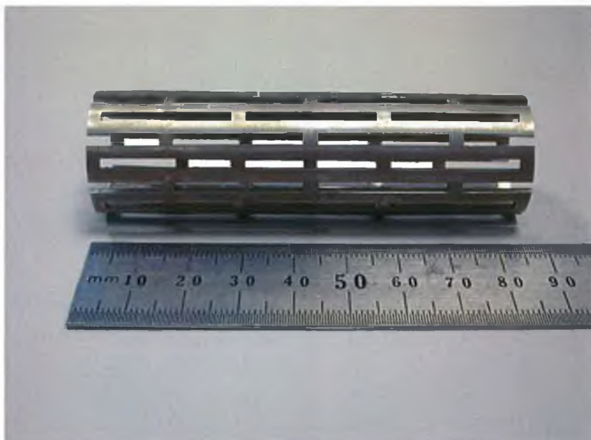
Figure 6.5: Design 3 (20 % decrease in width of the slot)
