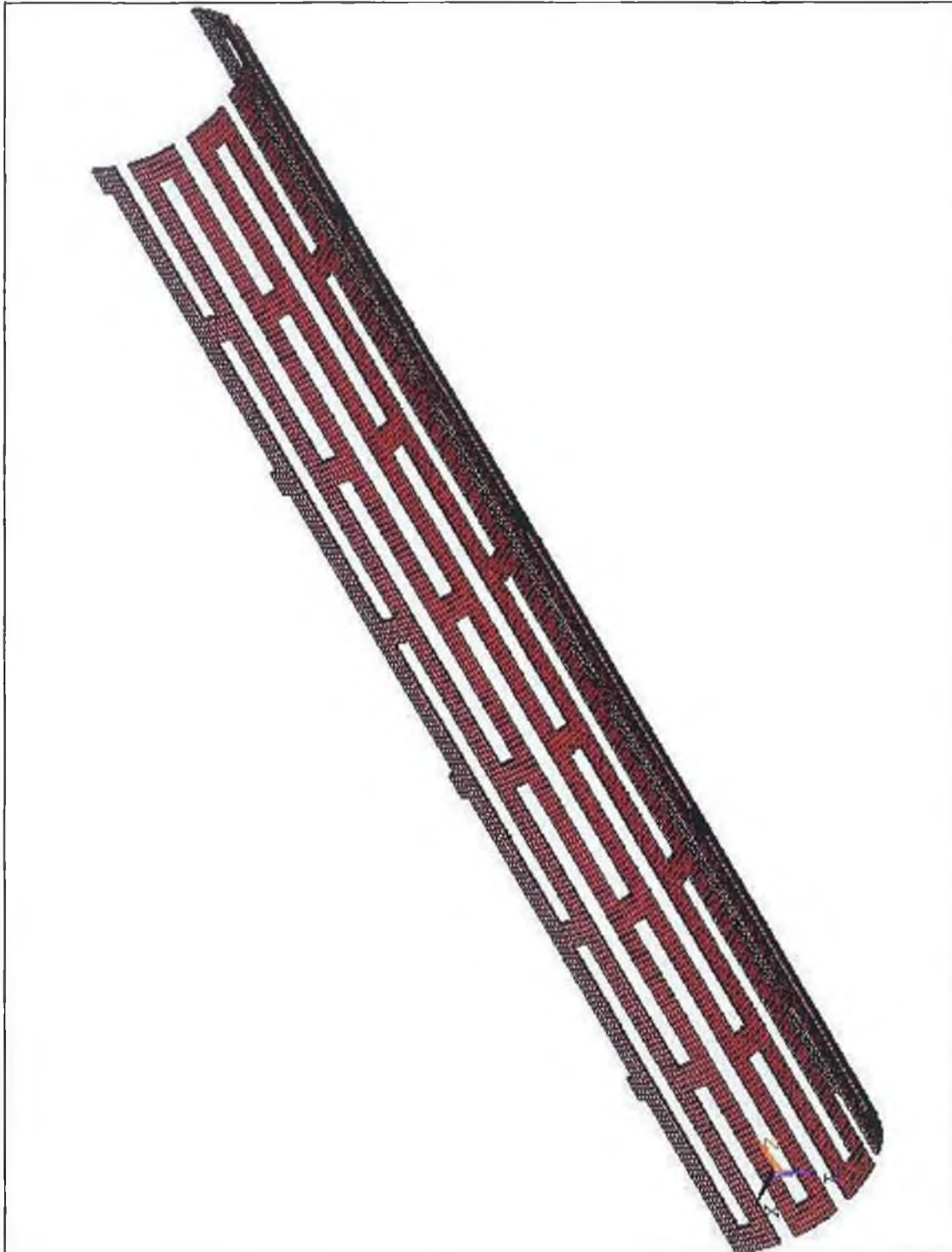
Figure 4.1: Finite element model of half of the stent
