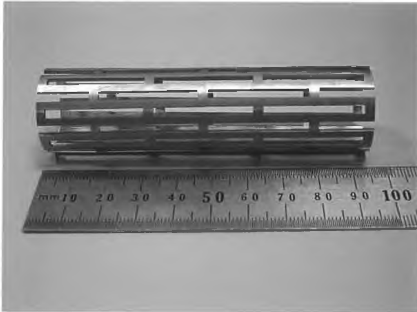
Figure 6.6: Design 4 (10 % increase in length of the slot)
