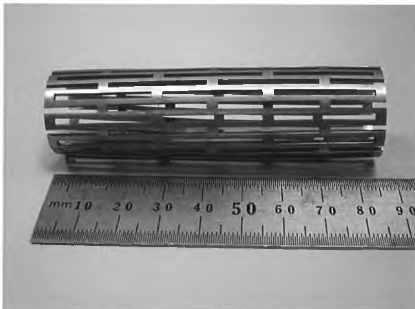
Figure 6.7: Design 5 (50 % increase in the number of slot)
