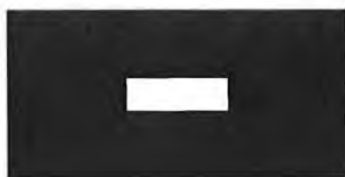
Figure B.1: Photomask used to define the SU-8 template for the fabrication of the PDMS flowcell used during the pH sensing experiments described in Chapter 7.
