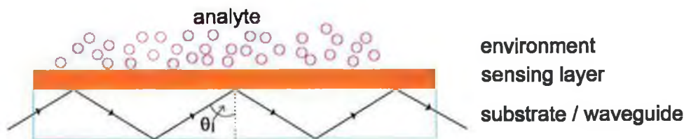
Figure 1.3: A multimode planar waveguide-based sensor.
