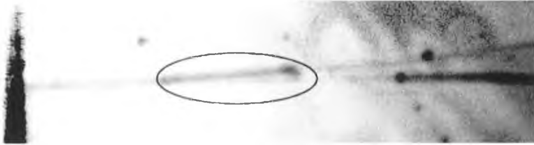
Figure 8.9: CCD image of light coupled from red laser diode to micromoulded Y-splitter. Double-exposed region at junction circled.
