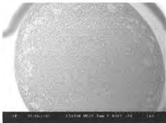
Figure 5-7: PPY formed on BAW surface using 0.1M \text{FeCl}_3 as oxidant
