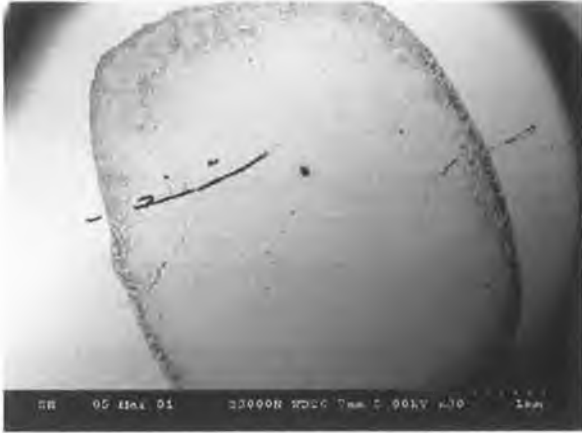
Figure 5-11: SEM image of PPY coated BAW after vapour deposition
