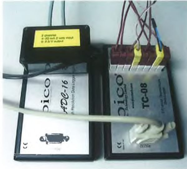
Figure 2.17: TC-08 signal converter and ADC-16 with 4-20 mA converter
