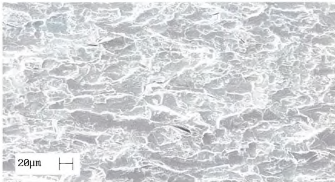
Figure 4.58 Base metal fractograph showing distribution of brittle cleavage facets, which occurred in synthetic seawater (-1040mV SCE).
