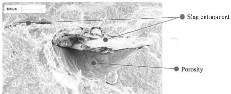
Figure 4.13 SMA fracture surface
