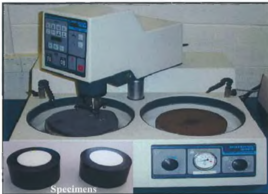
Figure 3.15 The Buehler Motopol 2000 Semi-Automatic Specimen Preparation unit. [33]
