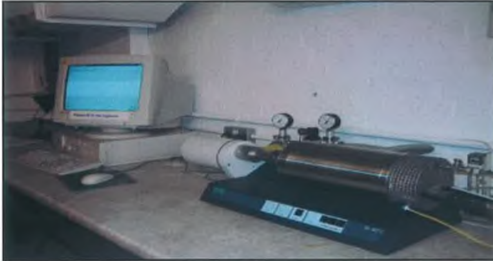
Figure 3.22 The dilatometer system used for thermal treatment.
