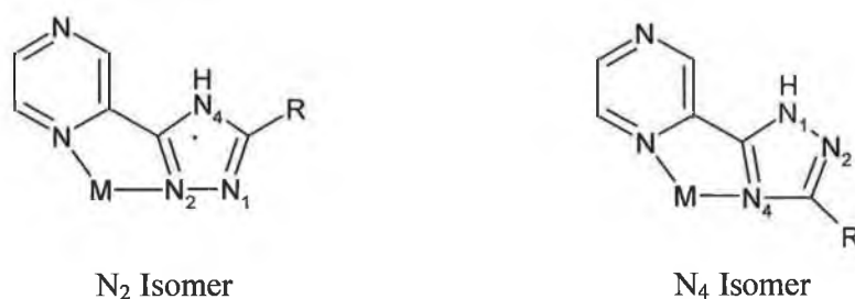
Figure 3. 6 The two possible modes of coordination of a metal centre to HRpztr.
