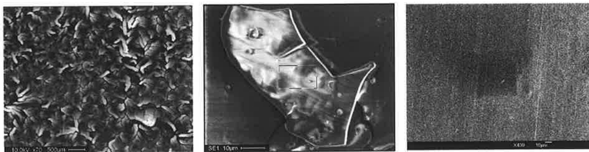
Figure 55 SEM image of mixed oxide coating after immersion in biological medium, deposited (a, b) without adhesion layer and (c) with SiO x adhesion layer
