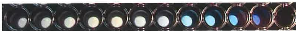
Figure 2.10 200 \mu L aliquots of increasing concentrations from 0.5 \mu M-20.5 mM of BCG at pH 7 in a 96 plate well.
