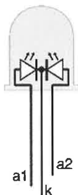
Figure 1.23 Schematic of Tri-colour LED [68].
