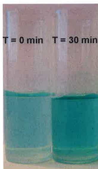
Figure 3.7 Photograph of 0.5 \mu\text{M} malachite green-molybdphosphate complex at (A) T = 0 minutes and (B) T = 30 minutes.
