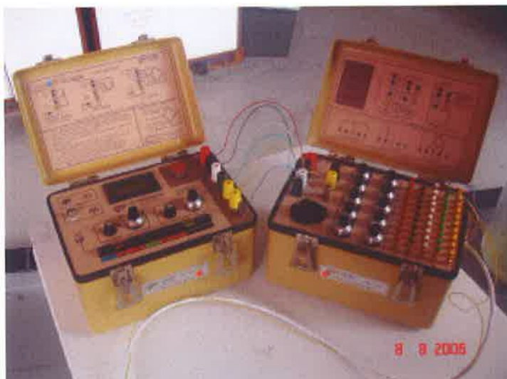
Fig. 4.9: Photograph of the digital strain indicator and the balance unit.
