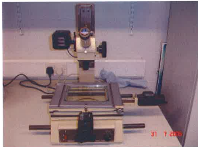
Fig. 4.14: Photograph shows the optical microscope used to measure the bead geometry.
