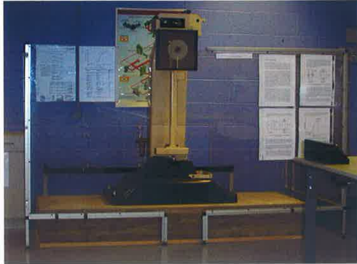
Fig. 4.22: Photograph of the standard ASTM universal pendulum impact tester.
