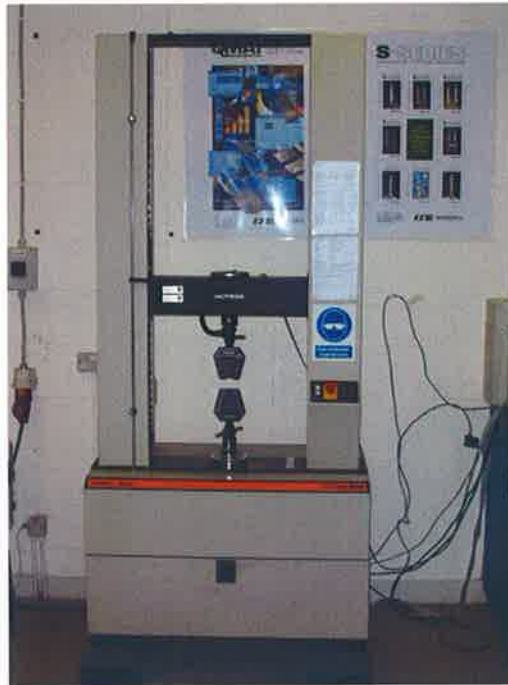
Fig. 4.16: Photograph shows the Instron testing machine.
