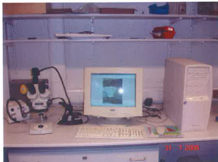
Fig. 4.16: Photograph shows the optical microscope and the software used to capture the entire weld-pool.
