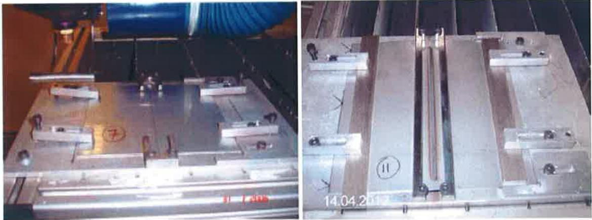
Fig. 4.2: Clamping the plates (a) butt-joint and (b) lap joint.
