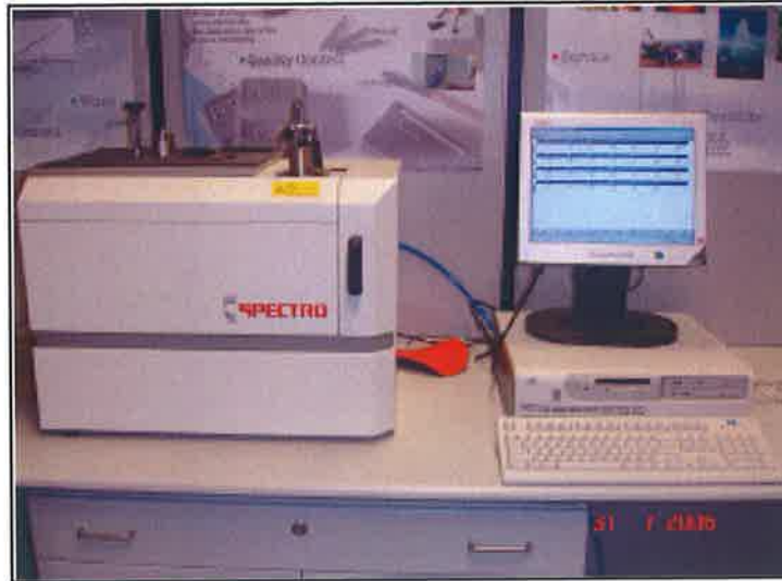
Fig. 4.1: Photograph of the Spectromax spark analyzer.
