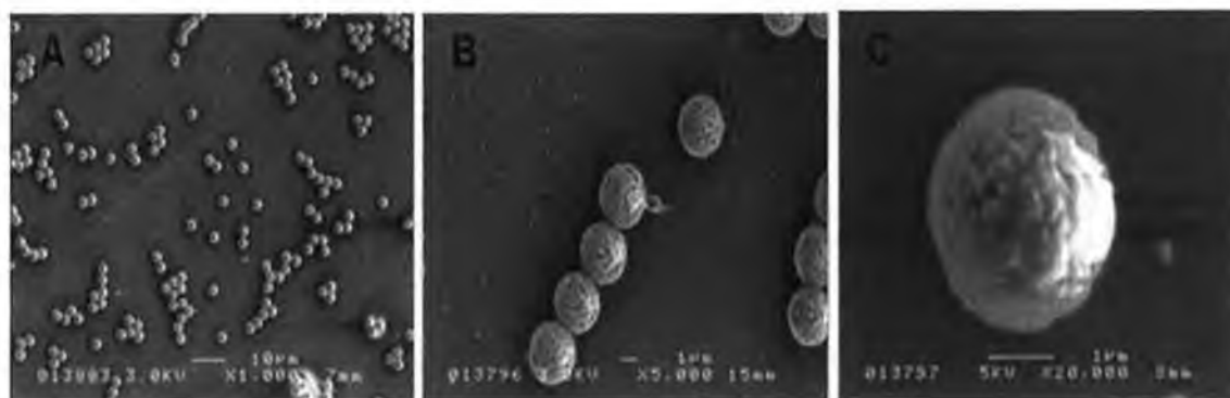
Figure 4.14. Scanning electron micrographs of streptavidin-coated magnetic beads (2,8 \mu\text{m} ) at (A) x 1k, (B) x 5k and (C) x 20k magnification. The MB sample was diluted with water and ultrasonicated for 20 min. prior the analysis. The size-dispersion is very narrow and that ensures a good quality of the assay results.
