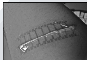
Fig 5: OECT with gel shown on a forearm.
