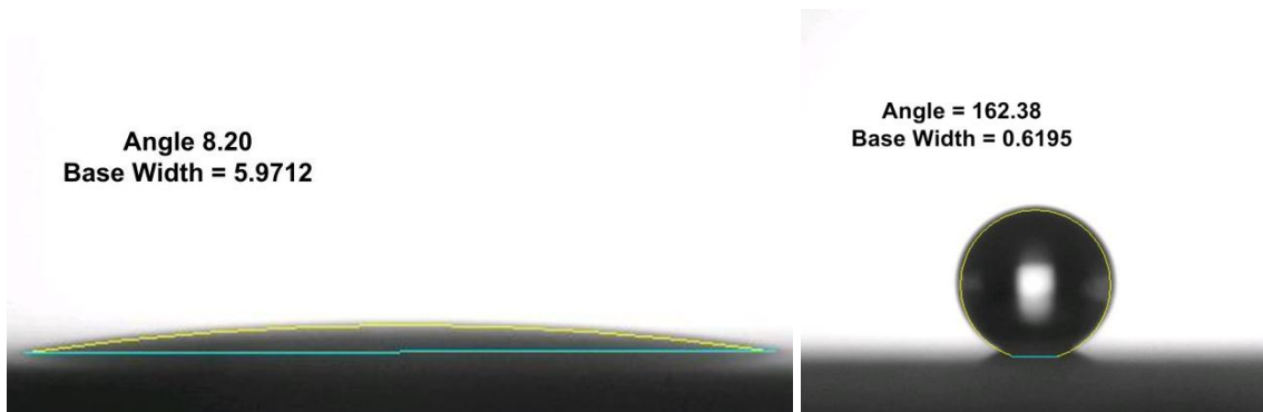
Figure 2-9: Super hydrophilic and super hydrophobic contact angles [95].
