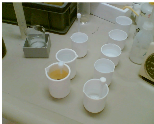
Figure 5.2 - PTFE Beakers used for holding cleaning liquids and etchants, arranged as an 'assembly line' leading from one step to the next.
