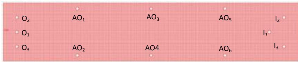
Figure 35: Layout of microfluidic chip with three main and six auxiliary outlets.
