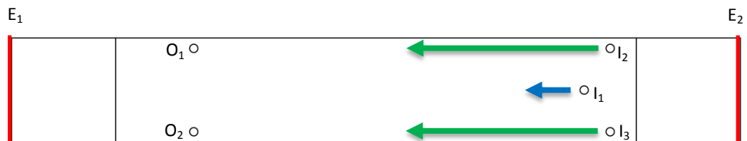
Figure 54: Schematic of the inlets and outlets and outlets used in the 2P-series experiments.
