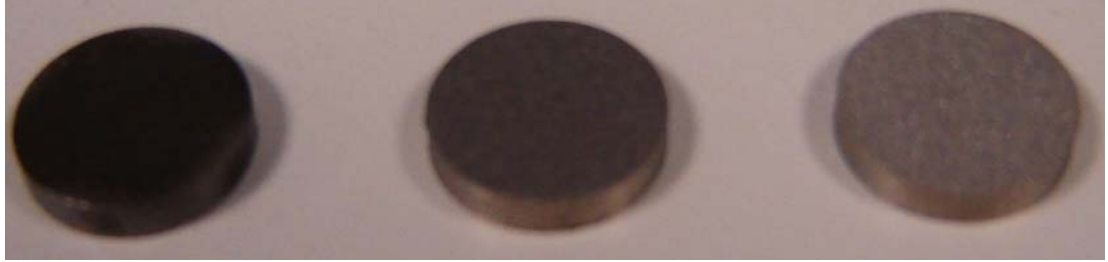
Figure 50: From left to right: orifice 4 used, orifice 3 used, bare Ti disc
