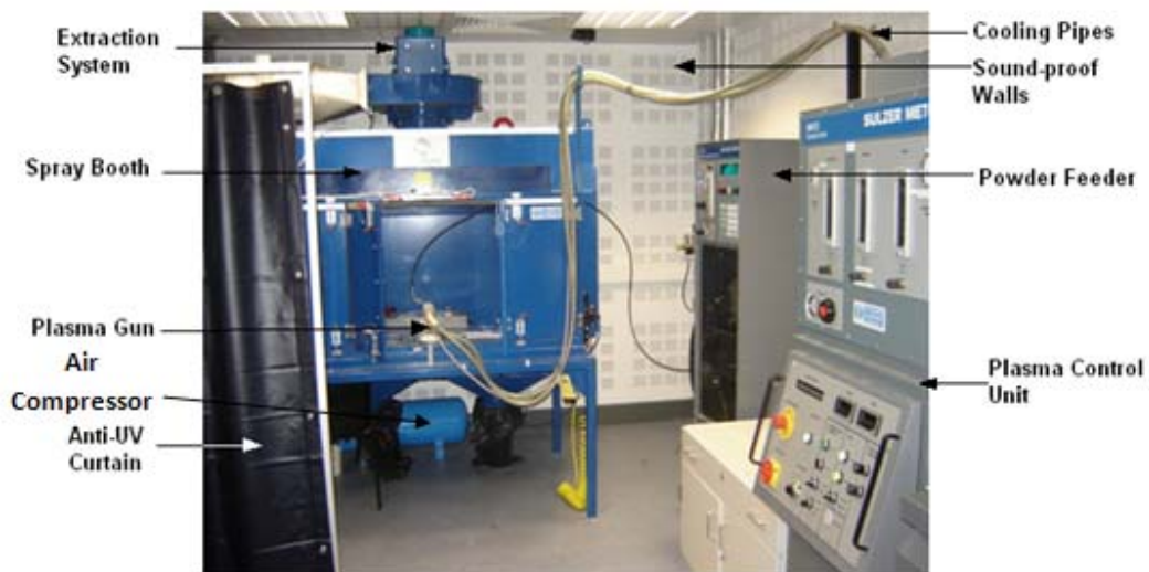
Figure 25: Plasma Spray System
