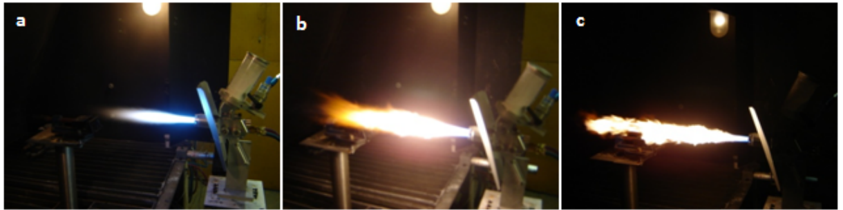
Figure 51: Plume appearance with: a) Neutral flame; b) powder orifice 3 used; c) powder orifice 4 used (excess powder)
