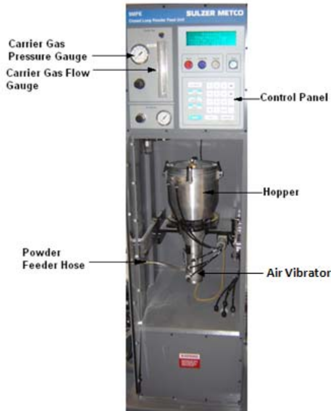
Figure 28: Sulzer Metco 9MPE Closed-Loop Powder Feeder
