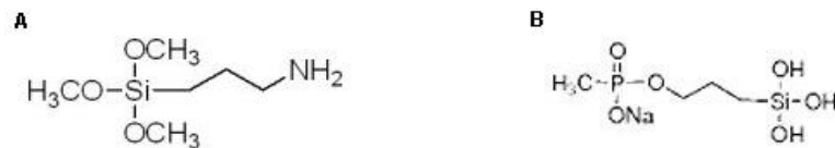
Figure 3.4: Chemical structure of A) APTMS, B) THPMP. APTMS is used to add amino groups \text{-NH}_2 on NP surface.
