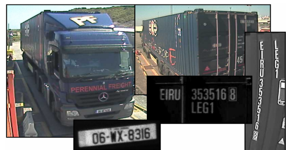
Figure 1. Freight-transporting vehicle with corresponding license-plates and container codes highlighted.
