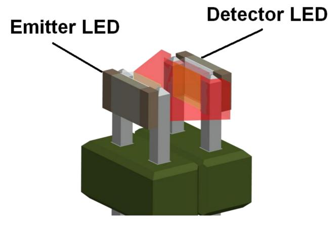
The colorimetric chemistry is immobilised on or between an emitter (forward bias), and detector LED (reversed bias), thus modulating the penetrating light.
