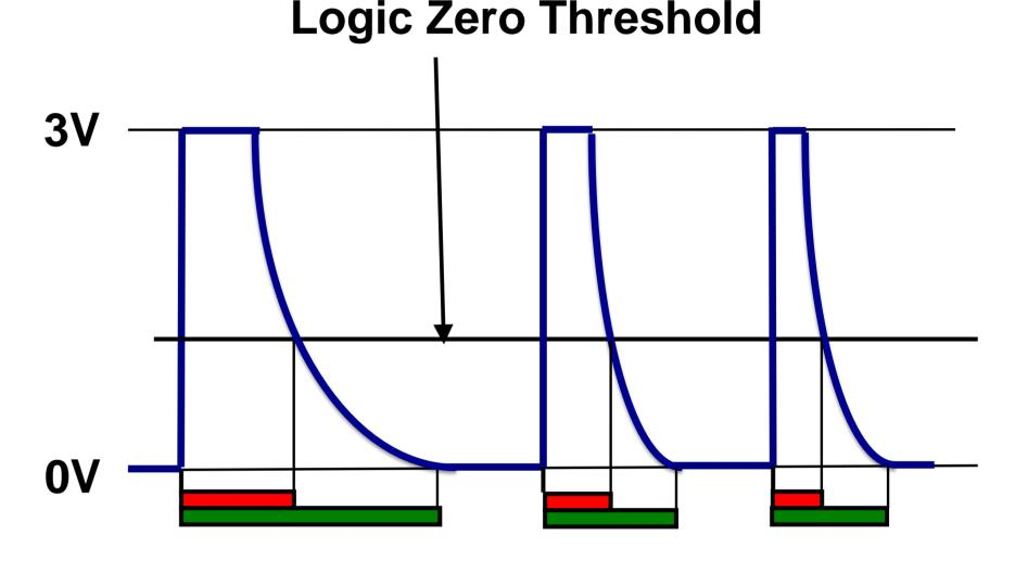
The microcontroller checks the amount of processor counts taken until the discharging capacitance from the reverse biased LED passes a logic threshold. This discharge is proportional to the light falling on it.
