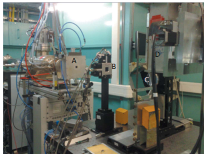
Figure 2 3D-XRDI experimental setup. 'A' is the fast shutter, collimating the beam to 10 \times 1 mm. 'B' is the final slit system to collimate the beam to 10 \text{ mm} \times 15 \mu\text{m} . 'C' is the sample holder containing a 200 mm wafer. 'D' is the CCD camera system.
